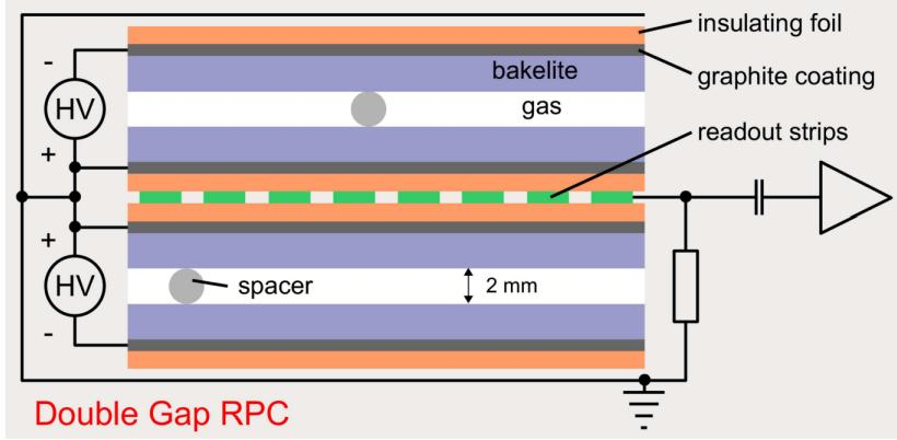
Figure 16. Cross section of a double gap resistive plate chamber [33]
