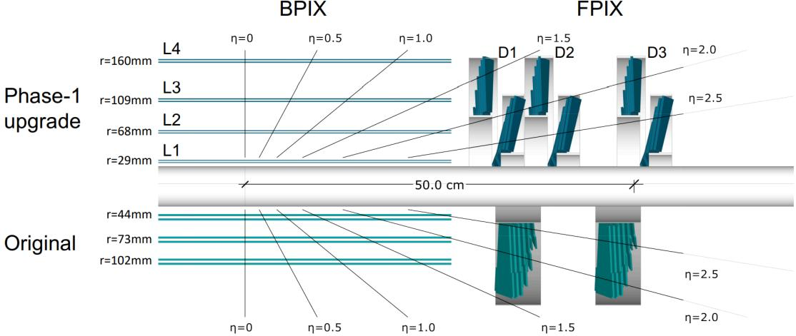
Figure 10. Comparison of the layout of the CMS Phase-1 pixel detector to the original detector. [29]
