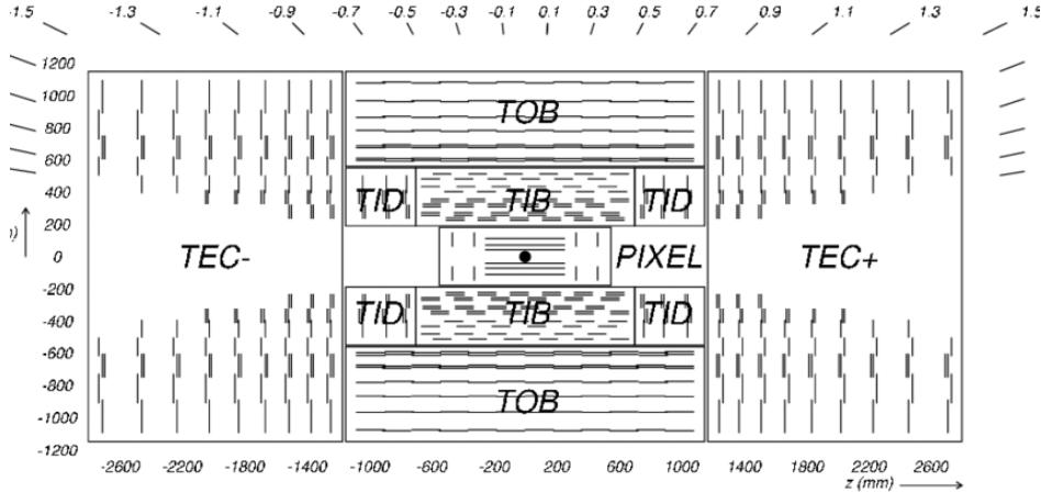
Figure 9. Schematic cross section through the CMS tracker. The silicon pixel detector in the center is surrounded by the silicon strip tracker parts: Tracker Inner Barrel (TIB) and Tracker Outer Barrel (TOB) detectors in the barrel region, Tracker Inner Disk (TID) and the Tracker End Caps (TEC) in the endcap regions. [20]
