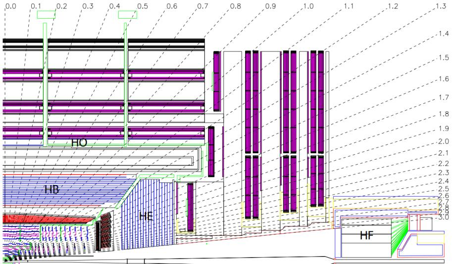
Figure 12. Longitudinal view of the CMS detector showing the locations of the hadron barrel (HB), endcap (HE), outer (HO) and forward (HF) calorimeters. [20]
