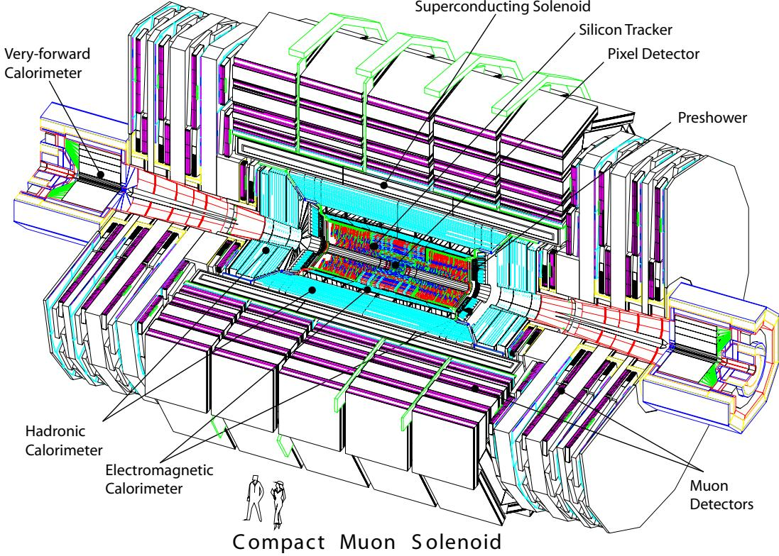
Figure 7. Schematic layout of the CMS detector. [26]
