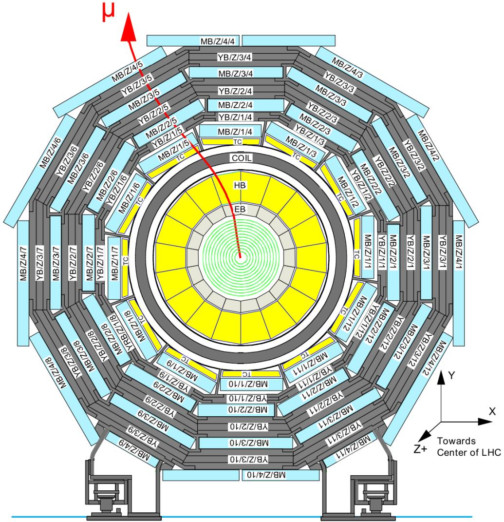
Figure 13. Layout of the CMS MB Drift tube chambers for one wheel of the iron yoke in  $r - \phi$  plane. The MB is divided into 12 sectors, which form four stations interleaved by the return yoke [30]
