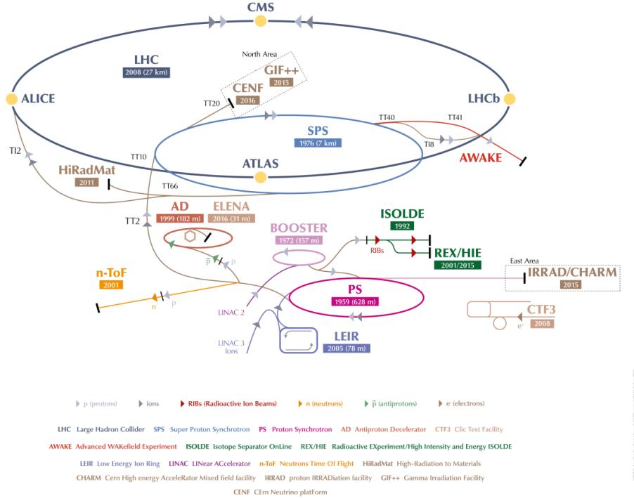
Figure 6. The CERN accelerator complex. The LHC is depicted as the dark blue line in a complex chain of particle accelerators, shown with its four main experiments. The smaller machines (pre-accelerators) are used in a chain to help boost the particles to their final energies before they get fed into the LHC. They are also used for smaller experiments.[23]
