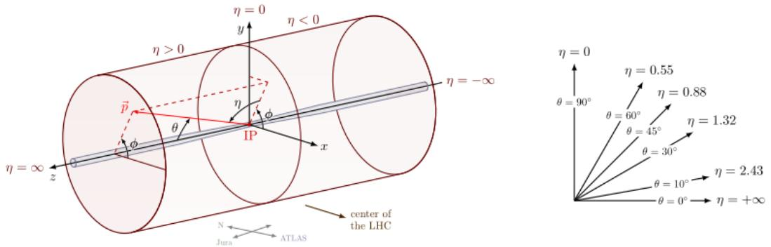
Figure 8. CMS coordinate system and pseudorapidity  $\eta$ . Here IP is the interaction point, which is the place where particles collide,  $\vec{p}$  describes the path a particle is travelling after the collision,  $\phi$  is the azimuthal angle, and  $\theta$  is the polar angle. [27, 28]
