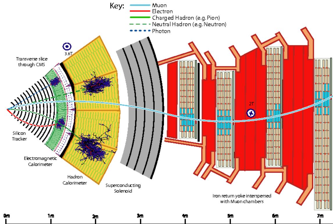
Figure 17. Schematic of the specific particle interactions in a transverse slice of the CMS detector. [36]
