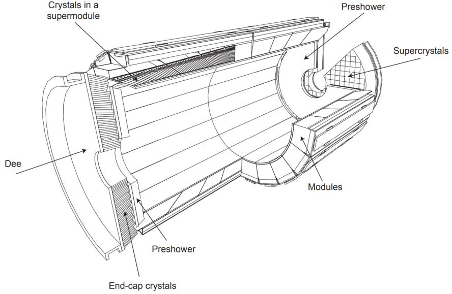
Figure 11. A 3-D view of the electromagnetic calorimeter [20]
