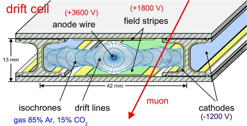
Figure 14. Cross section of a CMS drift cell with drift lines of electrons and isochrones [33]
