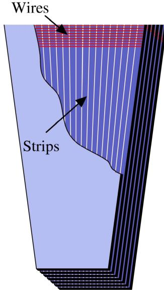
Figure 15. Sketch of a muon cathode strip chamber [33]
