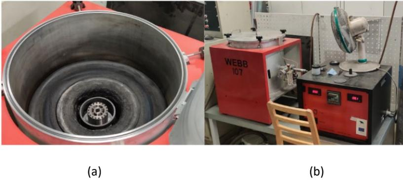
Figure 3.7. (a) Printed soft magnetic core in the annealing furnace, (b) full annealing setup with Webb-107 vacuum furnace. [136]
