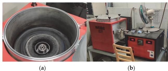
**Figure 6.** (a) Printed soft magnetic core in the annealing furnace; (b) full annealing setup of Webb-107 vacuum furnace.
