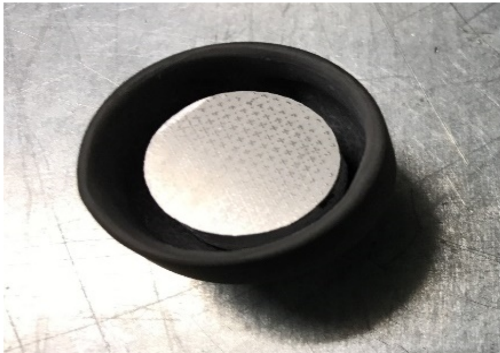
Fig.3.4 – SLM printed iron lattice SPS sample with aluminium
