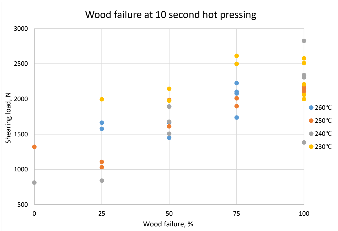
Figure 22. Wood failure with 10 second hot pressing.
