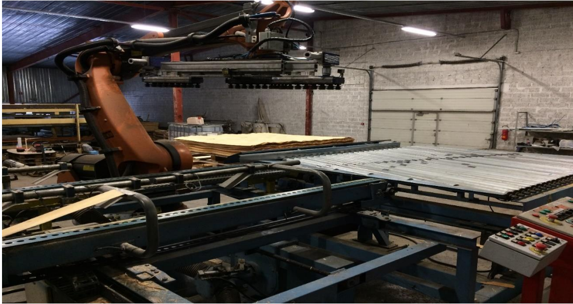
Figure 8. Veneer feeding machine followed by diagonal rollers.
