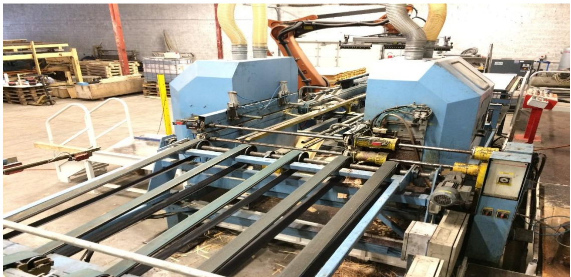
Figure 9. Circular saws followed by a conveyor belt.
