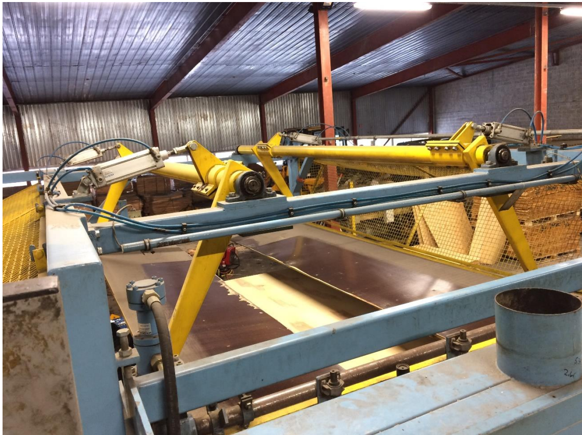
Figure 12. The scarf jointed veneer stacker.
