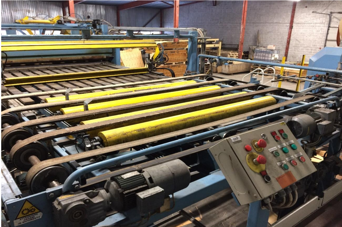
Figure 10. Cross conveyor belts followed by the scarf-jointing press.
