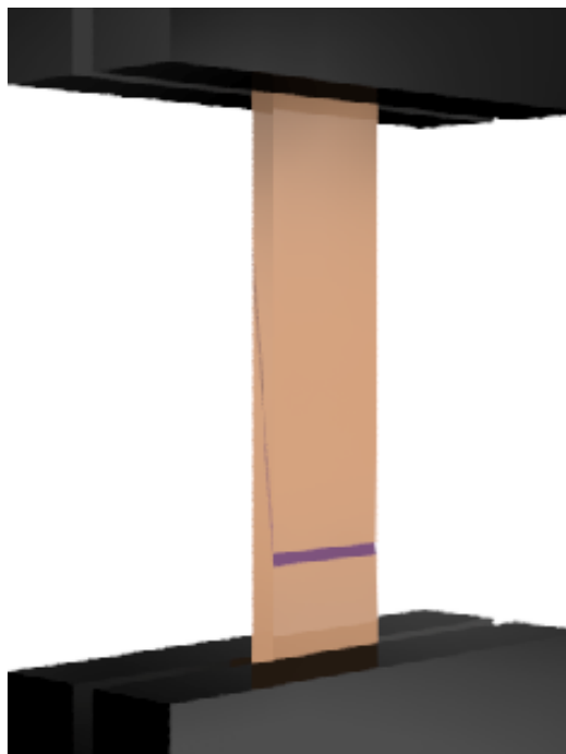
Figure 16. Instron crosshead clamps with a test sample inbetween.
