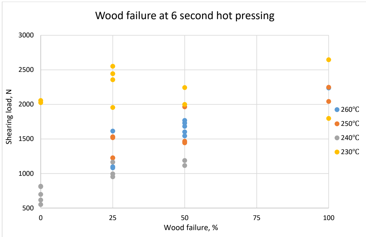
Figure 20. Wood failure with 6 second hot pressing.
