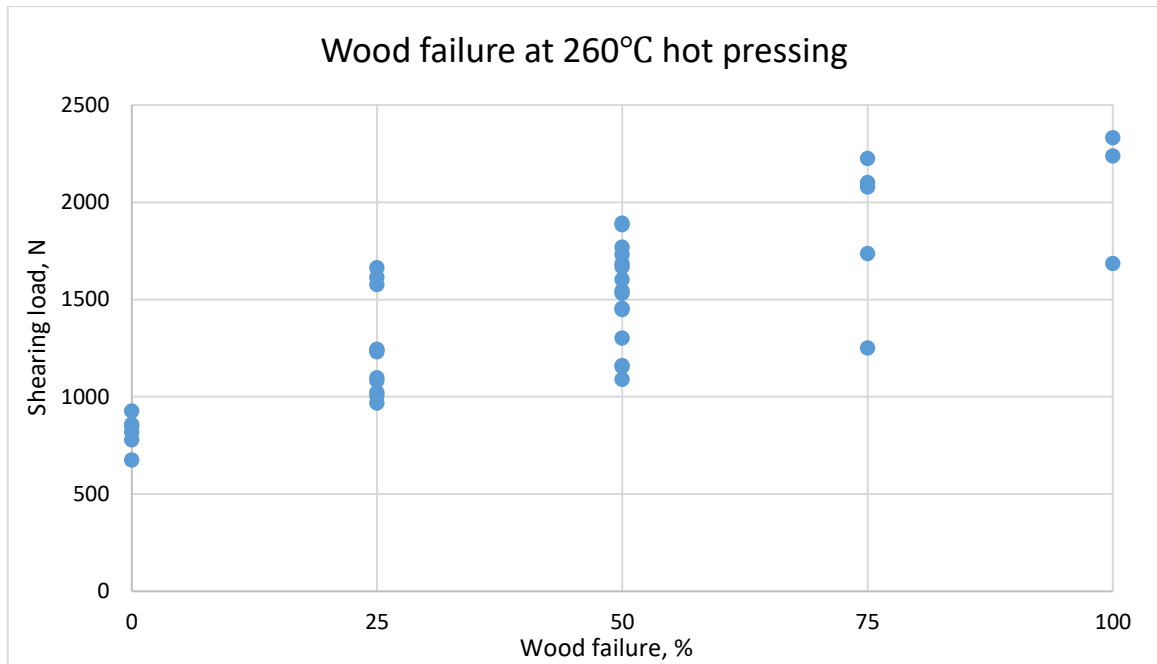
Figure 26. Wood failure of test specimen at 260°C hot pressing.
