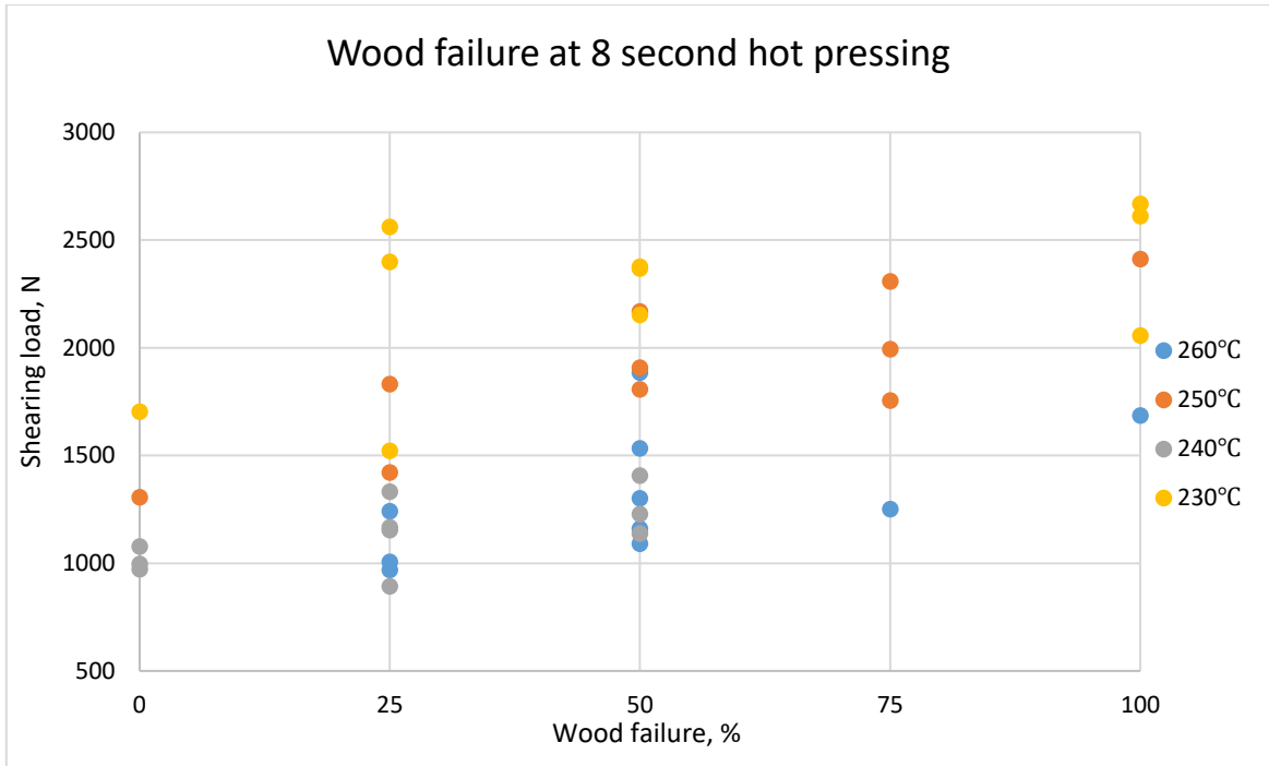
Figure 21. Wood failure with 8 second hot pressing.
