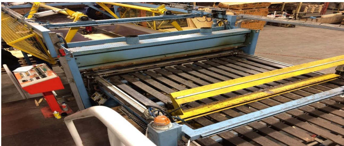
Figure 11. Scarf jointing hot press followed by the guillotine.
