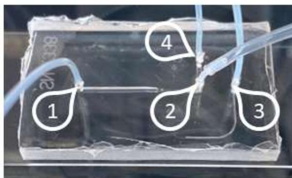
**Figure 13** PDMS microfluidic chip with tubes. 1 – sample inlet, connected to the oil syringe; 2 – droplet outlet, collecting droplets into a 5 ml tube; 3 – oil and surfactant mixture inlet, connected to the surfactant syringe; 4 – syringe for flushing the chip between samples and for stabilising pressure inside the chip, connected to an insulin syringe filled with HFE 7500 oil.
