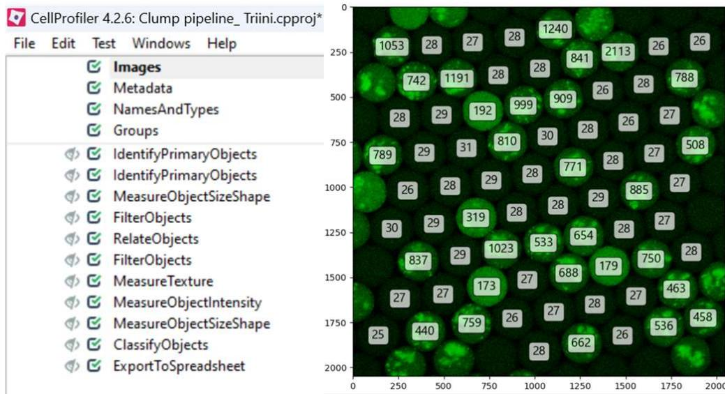
**Figure 16** Images from CellProfiler™. On the left is the pipeline used for the analysis after the threshold values were set. On the right is the workspace image from the pipeline used to set the thresholding values. The values show the degree of autoaggregation in droplets, the higher the number, the more autoaggregated bacteria in the droplets were.
