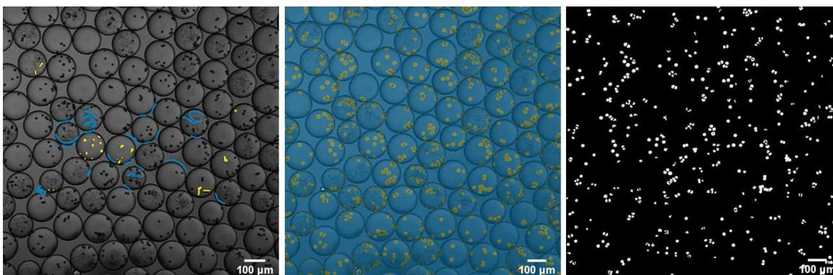
**Figure 15** Images from Ilastik training. On the left is an image from the training module: yellow and blue annotations were used to teach the program what are microbeads and what are not – yellow is for microbeads and blue is for everything else. In the middle is an image from thresholding module: program marks what it thinks are microplastics with yellow and everything else with blue. On the right is the Ilastik microplastic probabilities image used for CellProfiler™ analysis.
