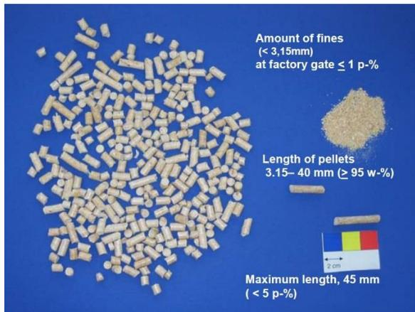
Figure 2.1 Dimensions of 8 mm wood pellets according to EN 14961-1[1]
