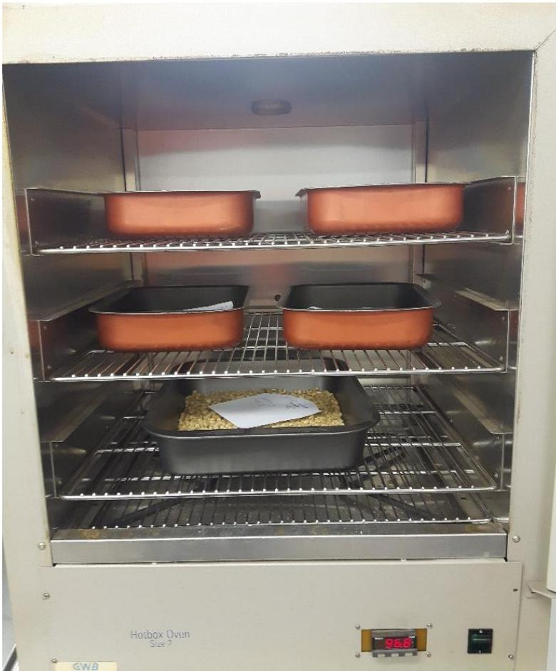
Figure 3.5 Arrangement of samples in Gallenkamp oven
