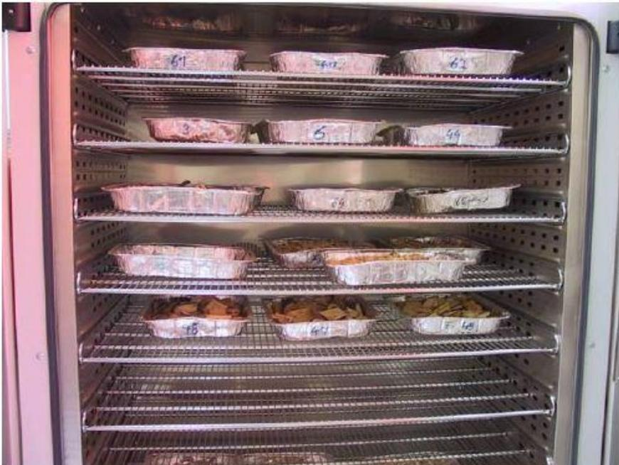
Figure 2.3 Drying of biofuel samples [14]
