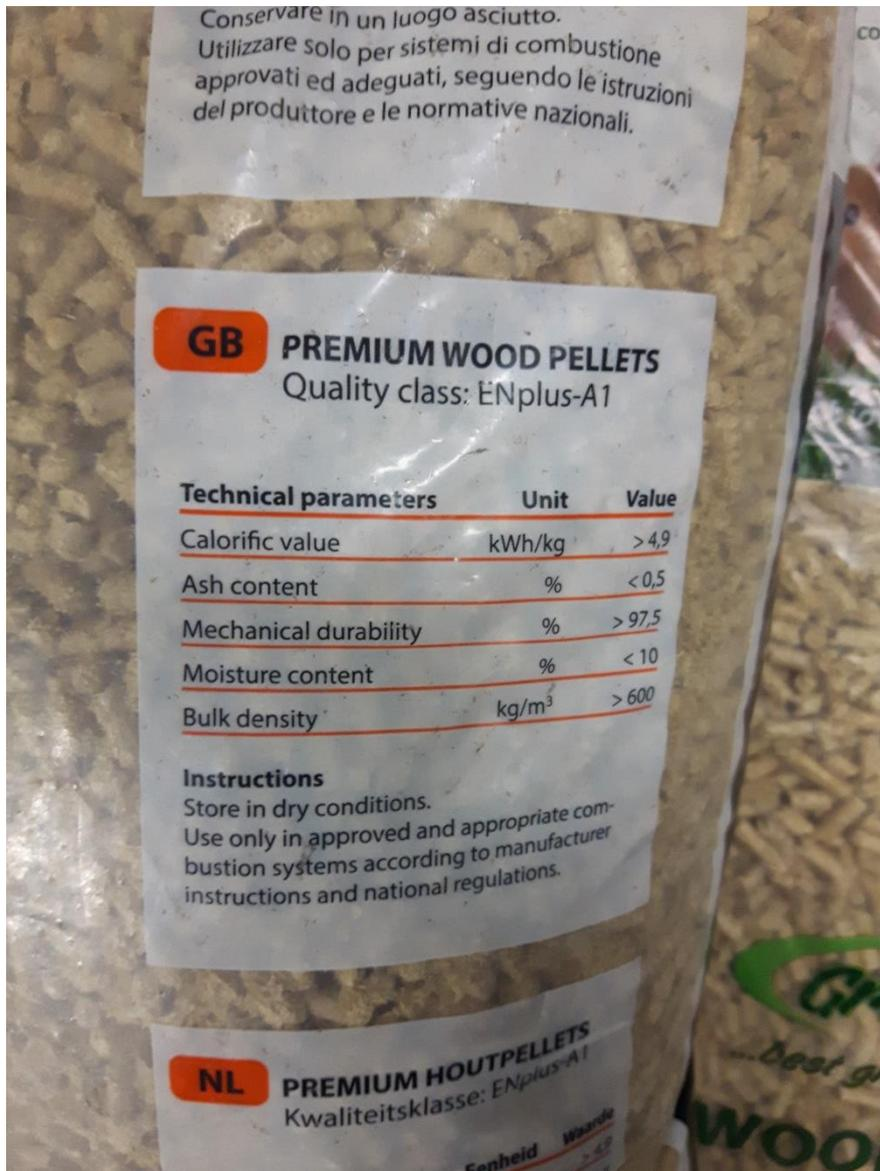
Figure 9.3 Technical parameters of pellets used
