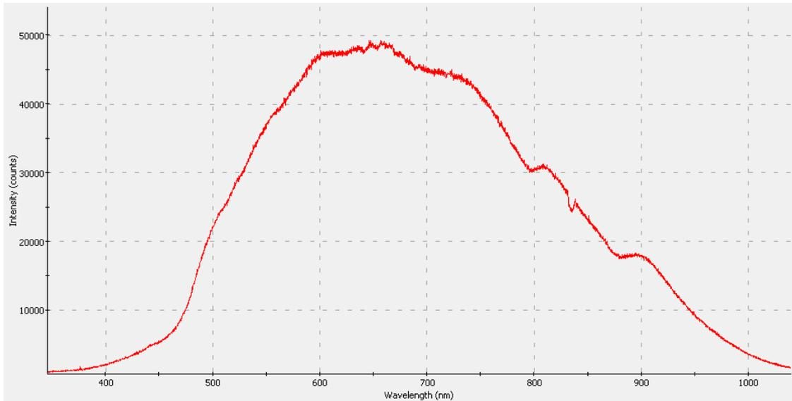
Figure 2 - 1. Spectrum of the Halogen lamp 12V 10W (Output power is 10W).
