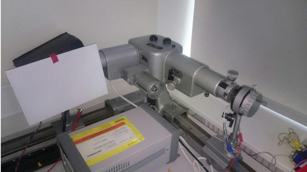
Figure 34. The setup for the wavelength response measurement. The platform with the LED is behind the white paper, under the black box.
