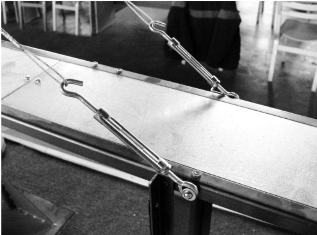
Figure 4.8 Anchoring of the cable-stay in the side span.
