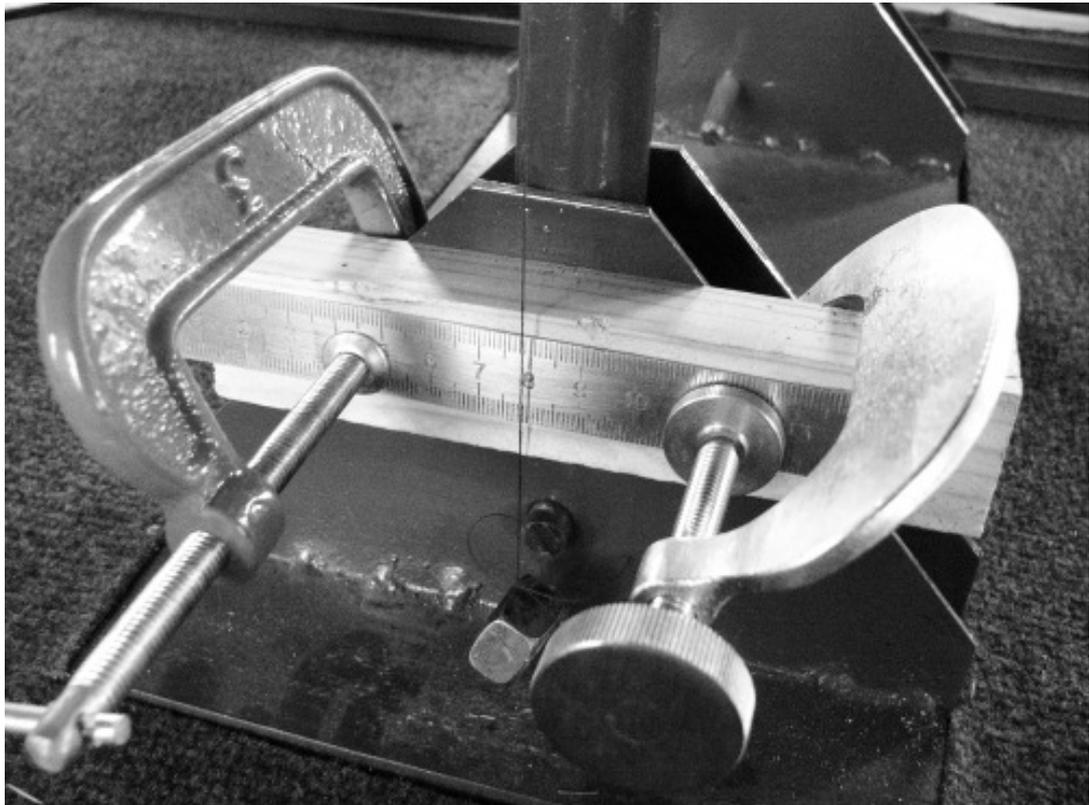
Figure 4.9 Measuring of horizontal displacements of the pylons.
