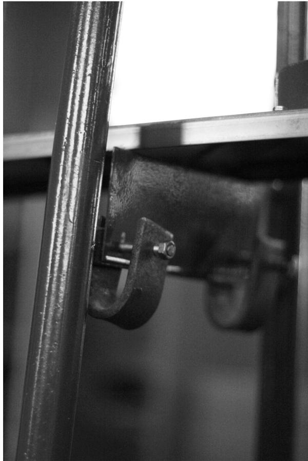
Figure 4.18 Supporting the stiffening girder in place of the pylons.
