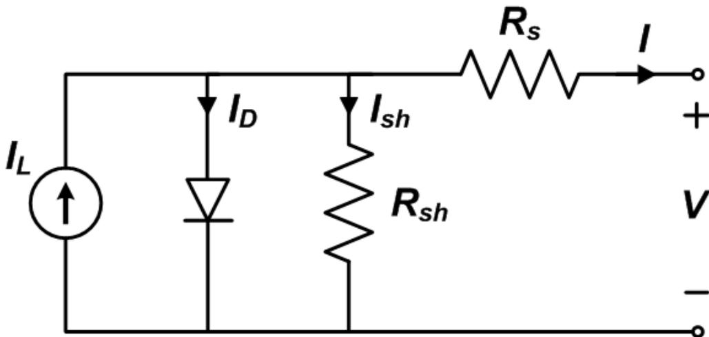
Fig. 1.4. Equivalent simplified circuit for solar cell
