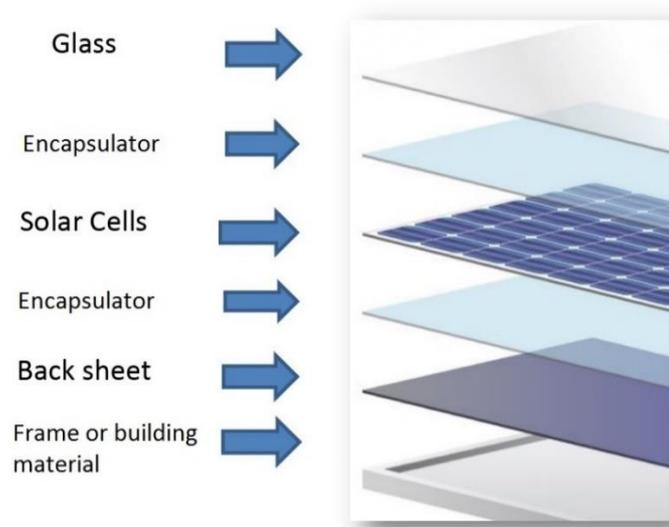
**Fig 1.8** Typical PV module structure
