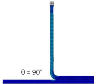
**Fig. 1.15** Peel stress test under  $90^\circ$  angle
