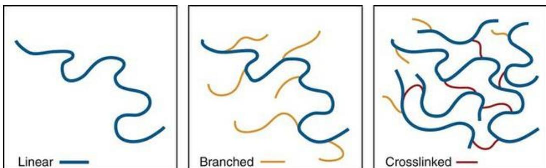
Fig. 1.12 Chain structure of linear branched and crossed-linked polymers
