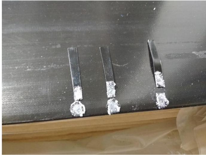
**Fig. 3.10** Shear stress results with Permabond TA4610. Surface treatment from left to right: plasma, alcohol, no treatment
