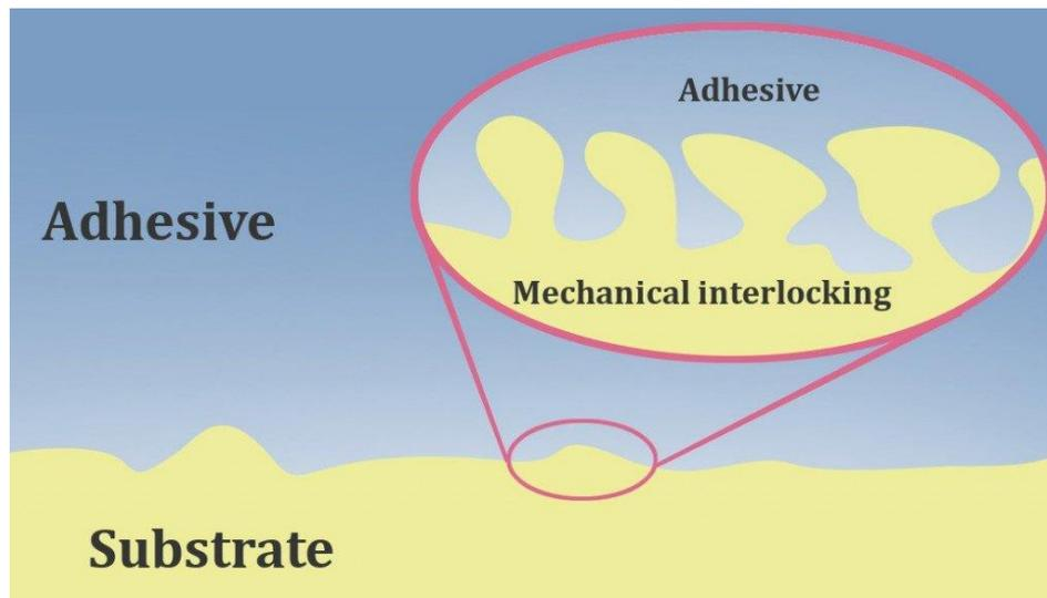
**Fig 1.11** Mechanical interlocking
