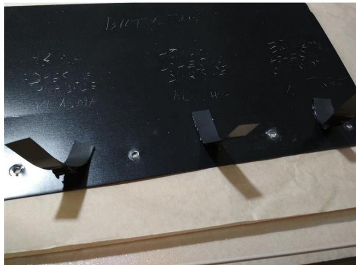
**Fig. 3.6** Peel test results for butyl tape. Surface treatment from left to right: plasma, alcohol, no treatment
