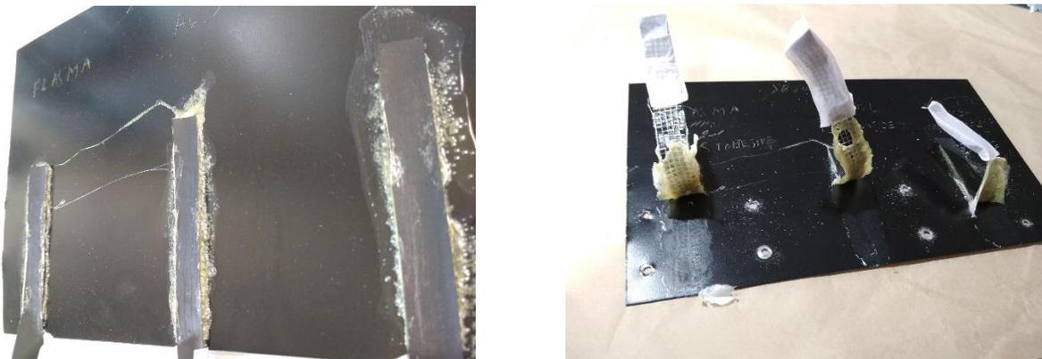
**Fig 3.3** Samples with SB 2444 adhesive before and after peel stress test. Surface treatment from left to right: plasma, alcohol, no treatment.
