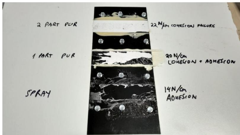
Fig. 3.2 Visual appearance of samples after peel stress test
