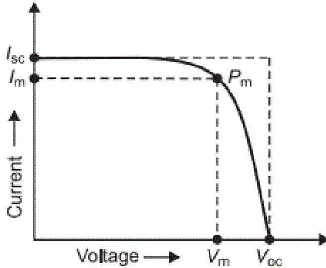
Fig. 1.5. Typical (I-V) curve with ideal parameters.
