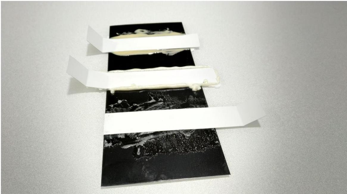
**Fig 2.1** Samples with PVF backsheet material
