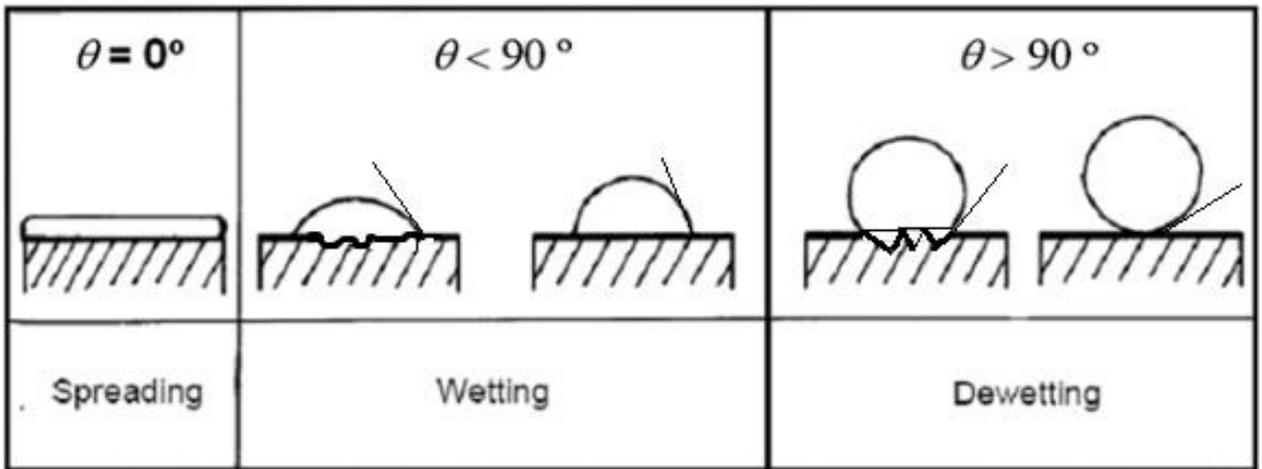
Fig. 1.10 Demonstration of good and poor wetting of substrate by adhesive.
