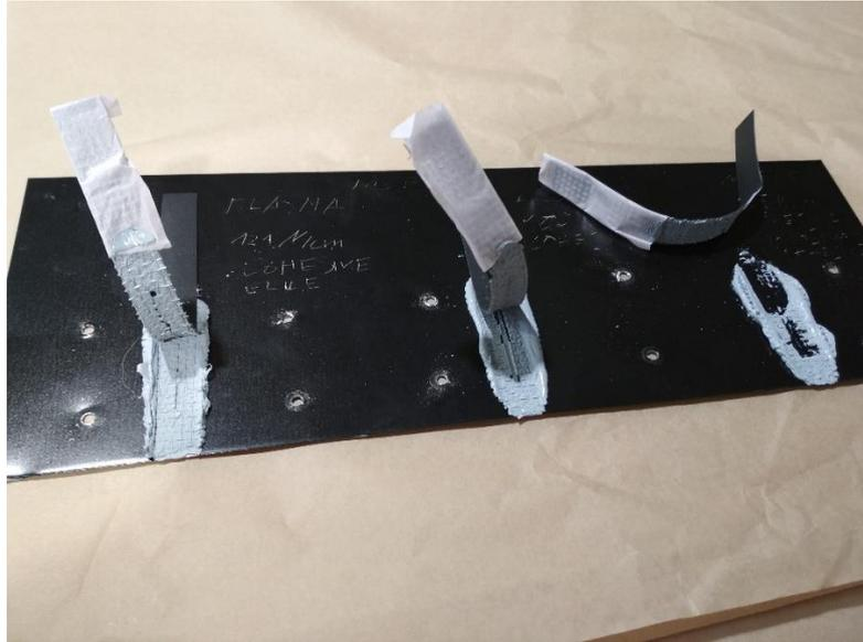
**Fig 3.7** Peel test results for Teroson 939. Surface treatment from left to right: plasma, alcohol, no treatment
