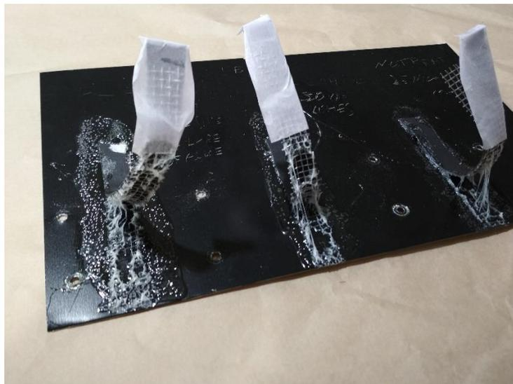
**Fig. 3.5** Peel test samples with SB 914 adhesive. Surface treatment from left to right: plasma, alcohol, no treatment
