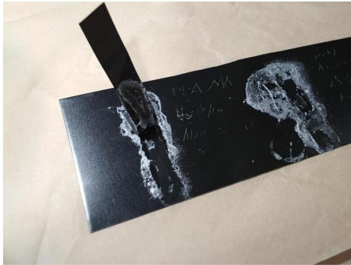
**Fig 3.4** Peel stress results of Teroson VR 5000. Treatment from left to right: plasma, alcohol.
