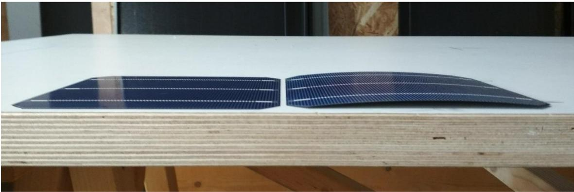
**Fig. 1.7** Difference in thermal expansion results in bending of solar cell.
