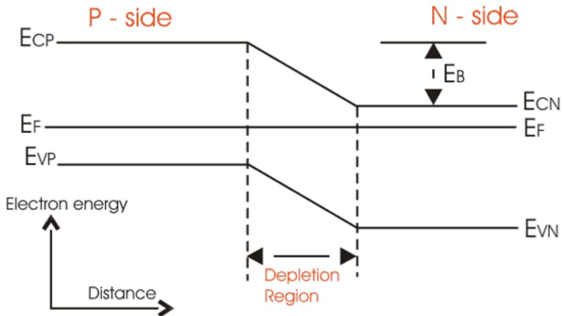
Fig. 1.3. Energy band diagram for p-n junction.
