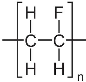
Fig. 1.13 Chemical structure of Polyvinyl fluoride
