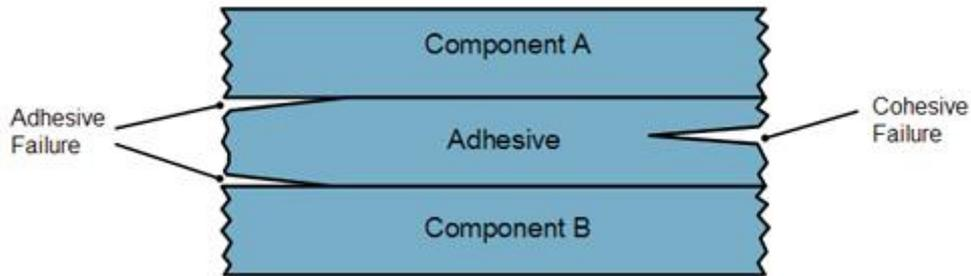
**Figure 1.9** Adhesive and cohesive failures
