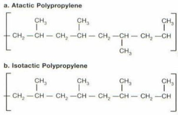
Fig. 1.14 Isotactic and atactic arrangements of polypropylene
