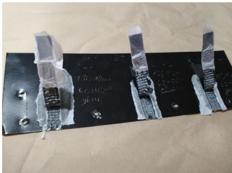
**Fig 3.8** Surface treatment peel stress results Permabond TA4610. Surface treatment from left to right: plasma, alcohol, no treatment
