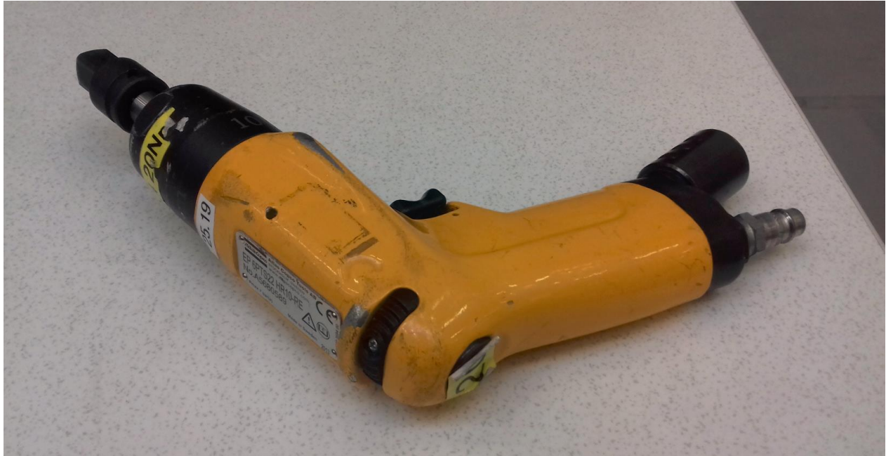
Figure 13. Typical air tool used on assembly line
