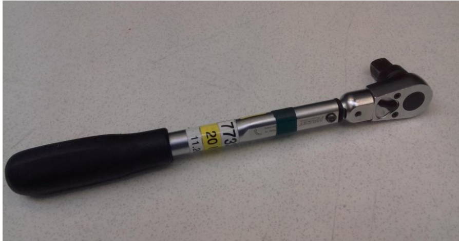
Figure 14. Typical racket head torque wrench used on assembly line
