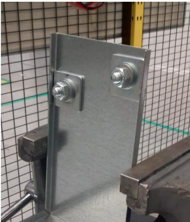
Figure 10. Test setup - front view – bolt, washer, metal plate, sheet metal plate
