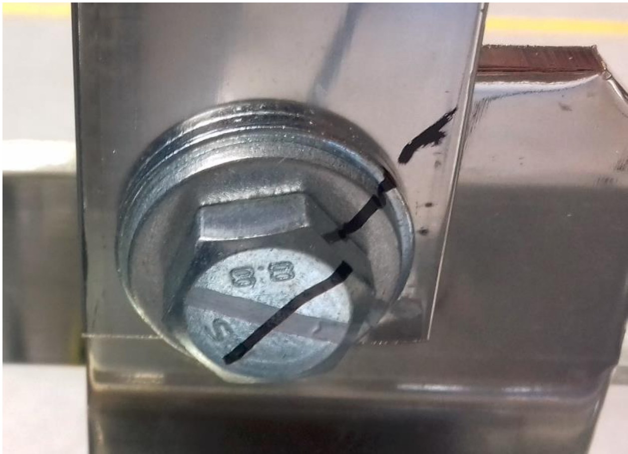
Figure 9. Marking of critical connection before and after double check
