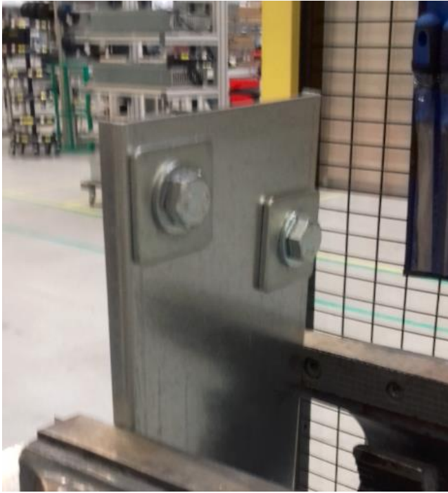
Figure 10. Test setup - front view – bolt, washer, metal plate, sheet metal plate
