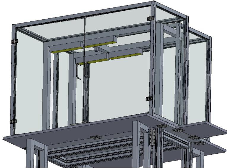
Figure 5.5 Location of the camera and light sources in the test bench.
