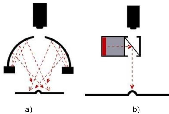
Figure 2.14 a) Dome lighting, b) Diffuse on-axis lighting [16]
