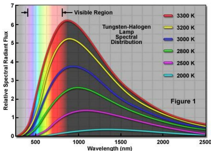
Figure 4.1 Spectral distributions of halogen lights [47]
