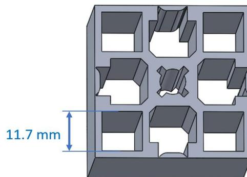
Figure 5.4 Extrusion of 45x45 G aluminium profiles of MiniTec.
