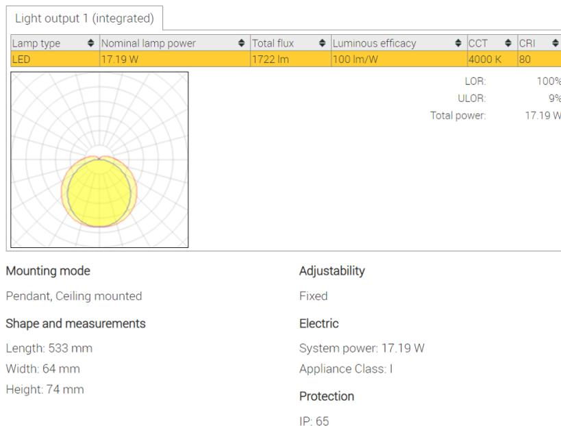
Figure 4.11 DSP52-18-041 Optima EM3 940 specifications from the ASTZ manufacturer [55]
