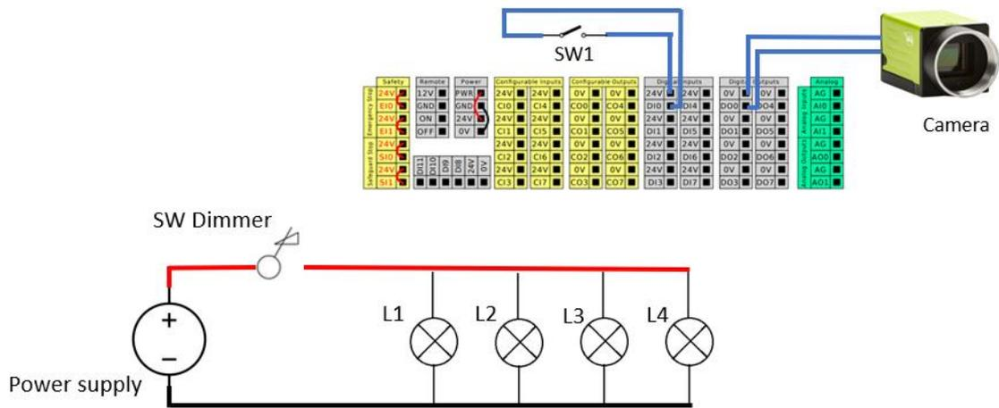
Figure 5.3 Electrical circuit for four halogen lamps
