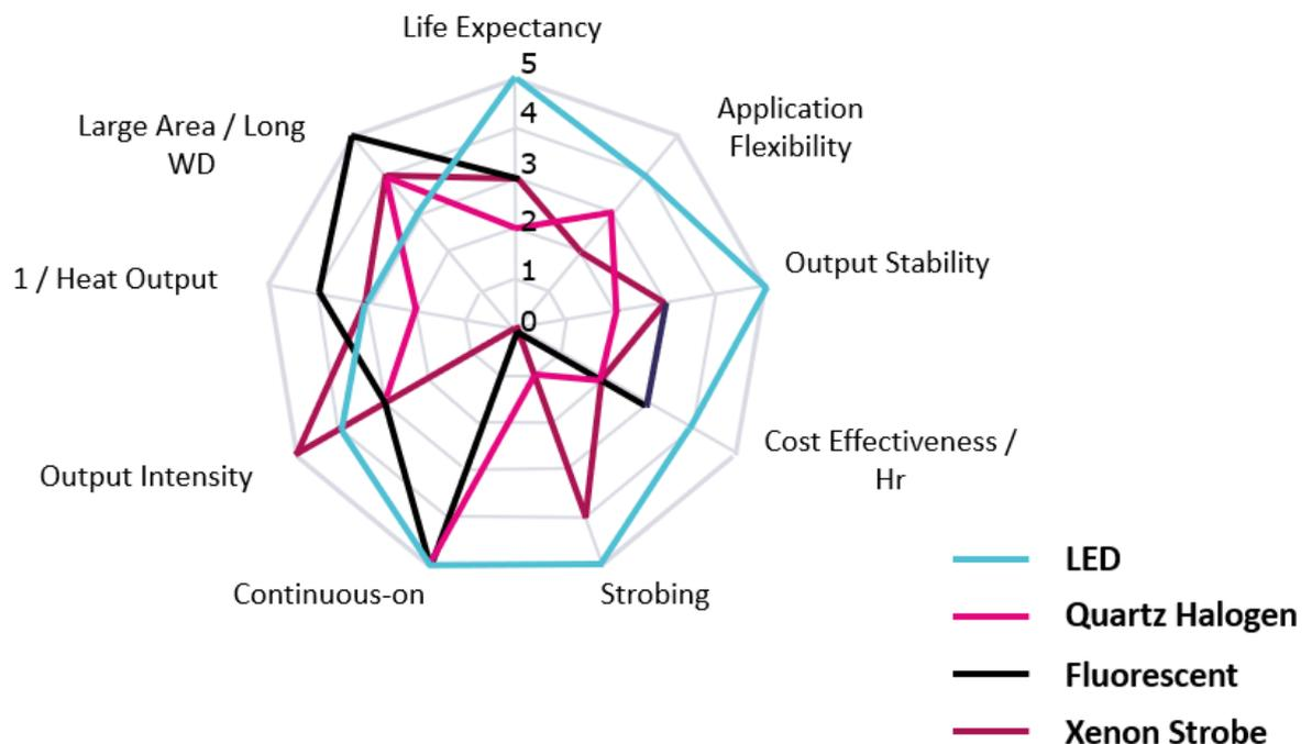
Figure 2.8 Comparative graph of illumination sources [16]
