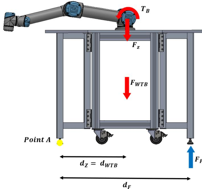
Figure 3.8 Internal forces of test bench for modified draft
