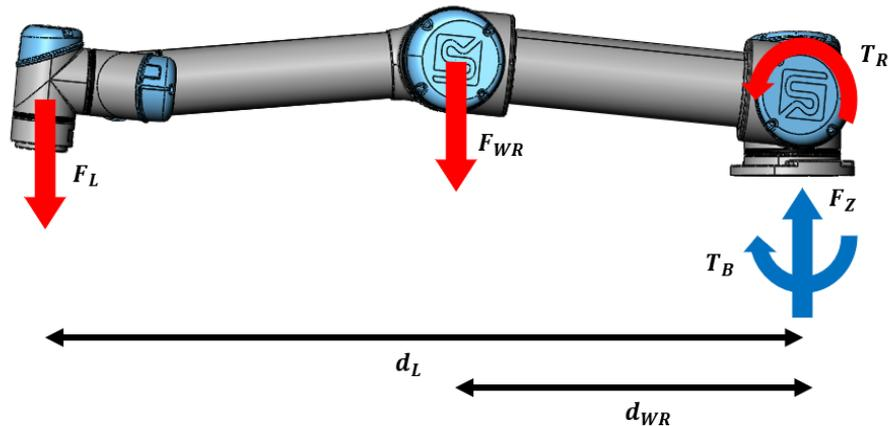
Figure 3.4 Internal forces of robotic arm
