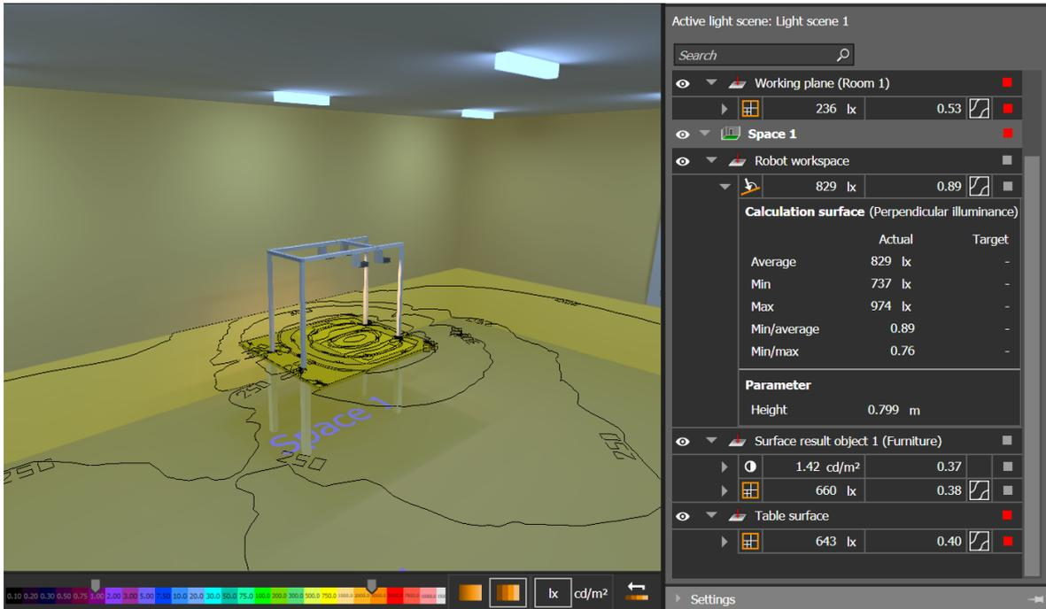
Figure 4.12 Results obtained when the light of the room is added
