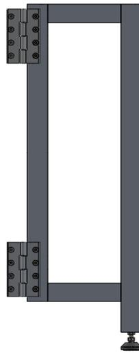
Figure 3.6 Legs for supporting the wings
