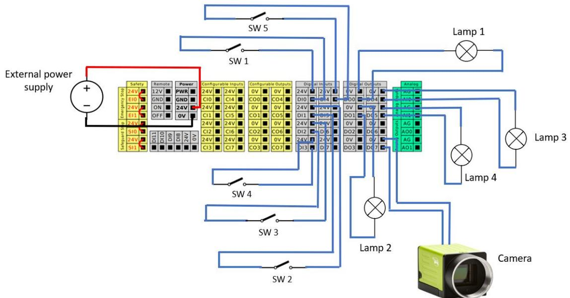
Figure 5.2 Electrical circuit for four HSI LED
