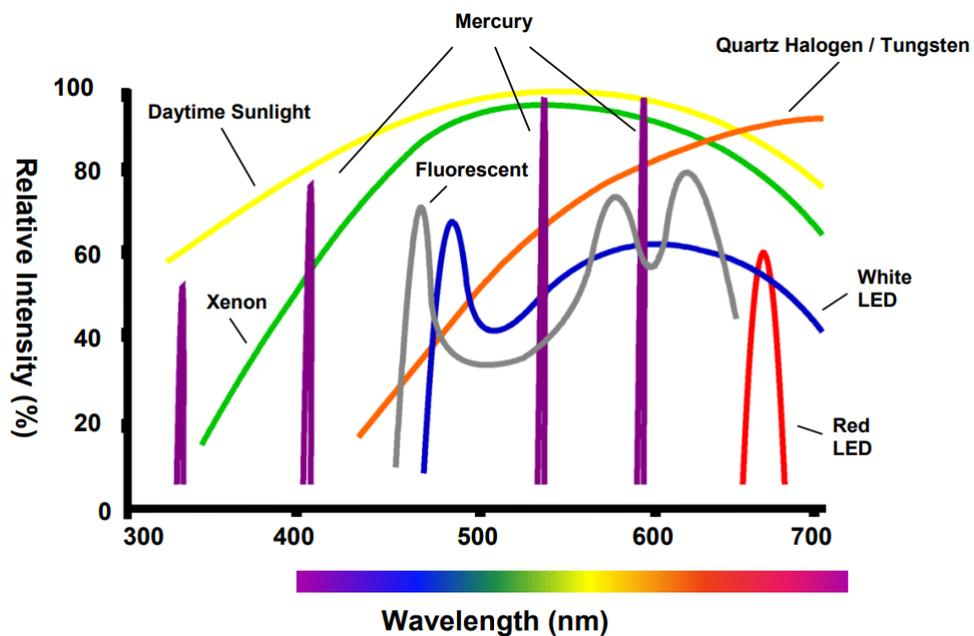
Figure 2.9 Wavelength vs Relative Intensity of light sources [16]
