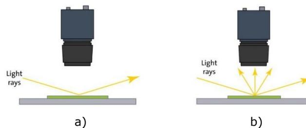
Figure 2.12 a) Dark field flat surface, b) Dark field imperfection surface [20]
