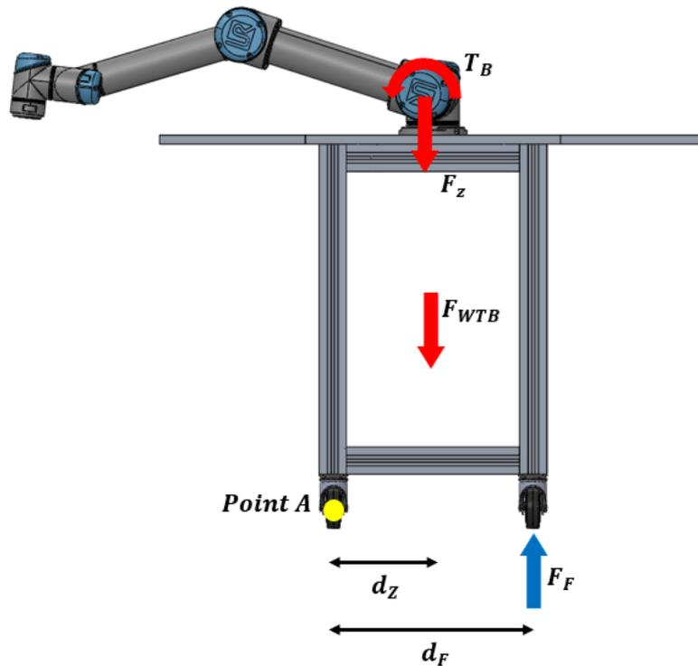
Figure 3.5 Internal forces of test bench for first draft
