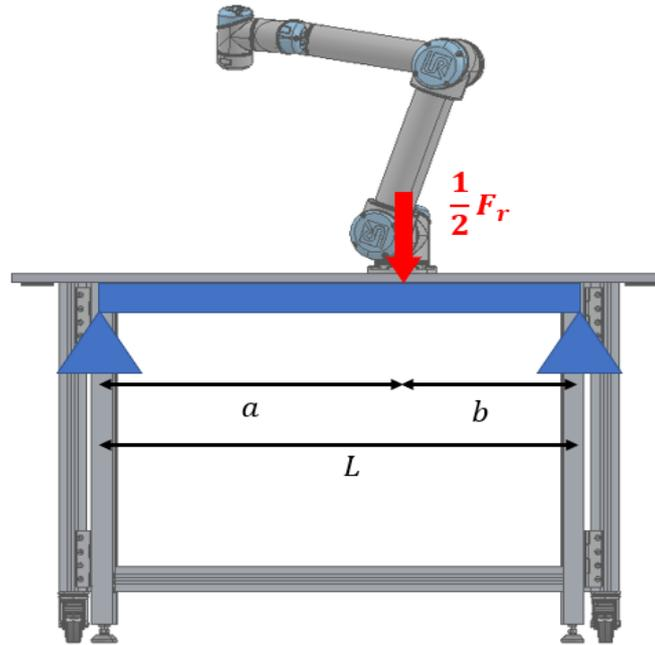
Figure 3.9 Scheme of forces to calculate deflection
