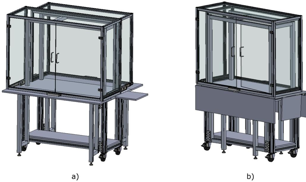
Figure 3.15 Final design where a) Full opened test bench, b) Closed test bench
