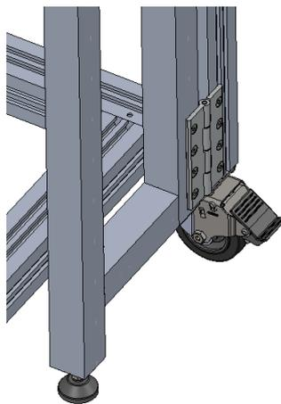
Figure 3.7 Retracted leg position
