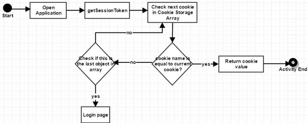
Figure 19 An Activity Diagram about the Logic behind Keeping the Section Alive.
