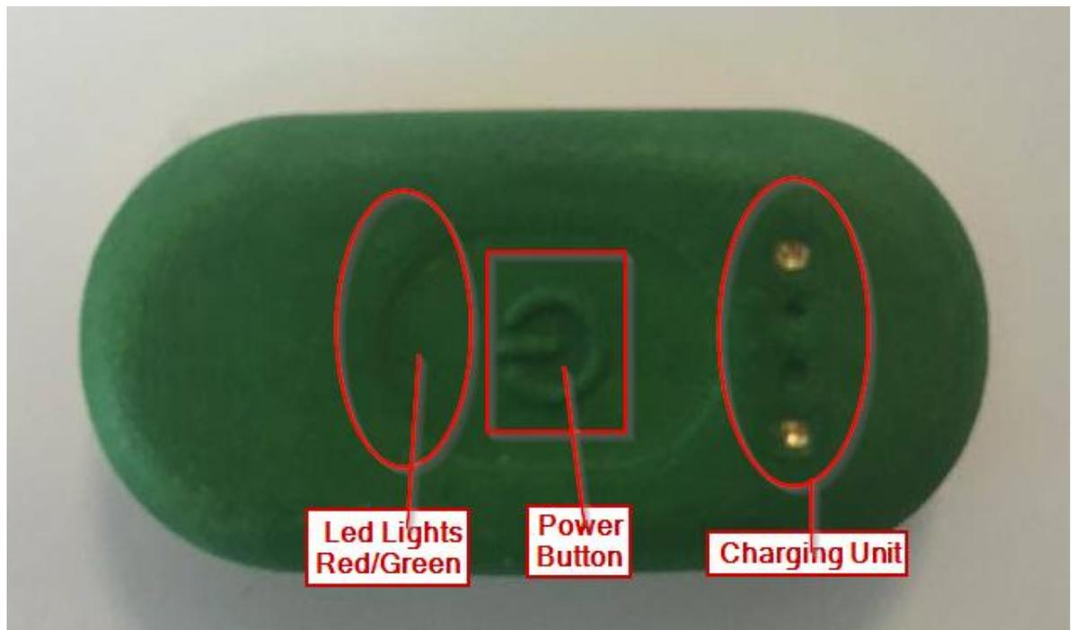
Figure 13 BLE Wearable Sensor.
