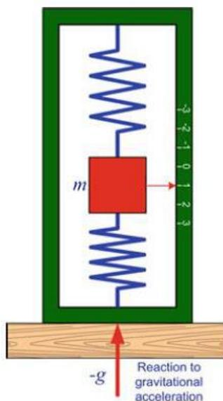
Figure 4 Gravitational force measurement of an accelerometer [10].
