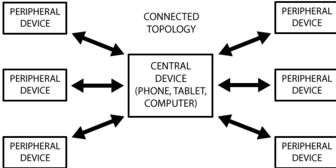
Figure 14 Network Topology BLE peripheral device and central device [36].
