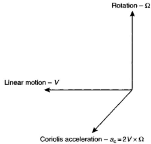
Figure 8 Coriolis acceleration which is generated by linear motion and rotation[15].
