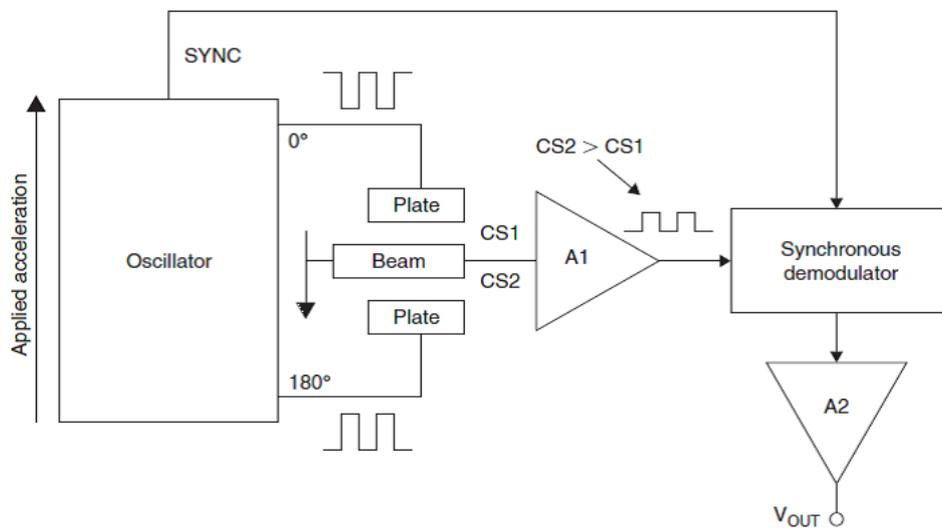
Figure 5 Working principle of a capacitive accelerometer [12].
