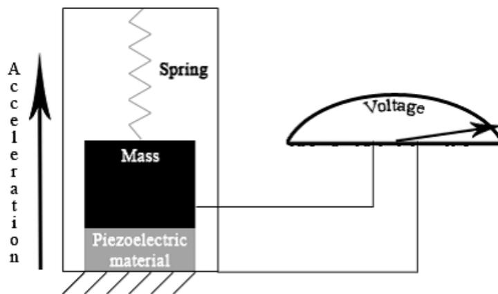
Figure 6 - Applied acceleration trigs voltage generation for piezoelectric material [8].
