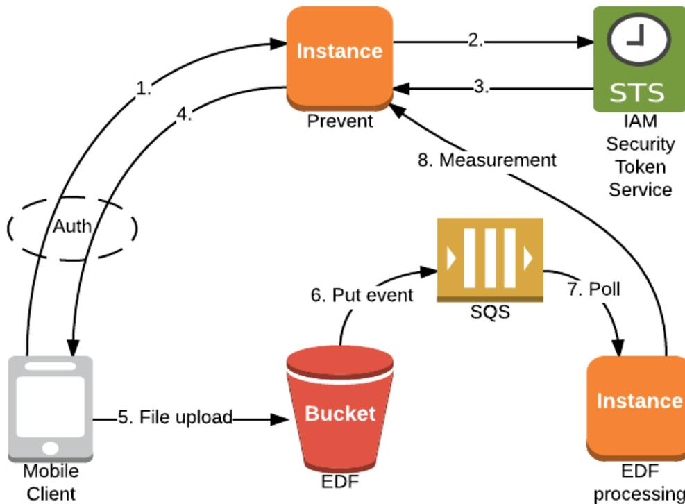
Figure 16 Visual demonstration for Backend Communication.
