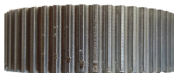
Figure 9. Example of pulley teeth cracks of the gearbox.
