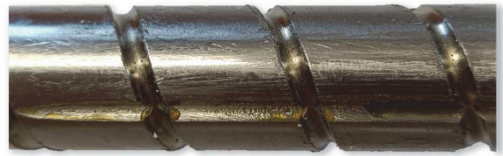
Fig. 2. Example of the heated worm of the screw transmission.
