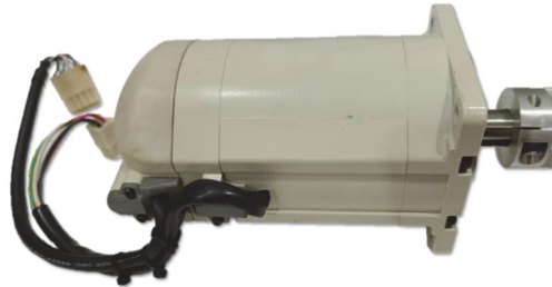
Figure 2. The servomotor used in a Hirata Cartesian robot.
