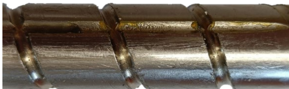
Figure 3.3. The example of the worm heating in the screw transmission. (previously published in article II)
