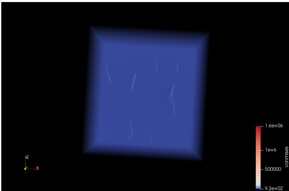
Figure 7. Von Mises stress visualization for the specimen reinforced with hooked fibers.
