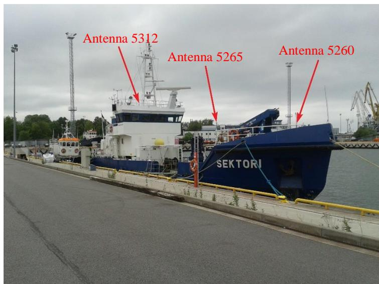
**Figure 3.1** Estonian Maritime Administration survey vessel “MS Sektor”. Red arrows point to the locations of GNSS antennas (see also Fig. 3.3).
