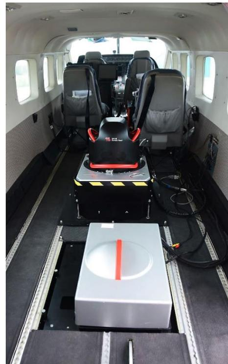
**Figure 4.2** Leica ALS50-II LiDAR System (in the left figure) and it placed on the survey plane (the foremost instrument in the right figure; survey plane in Figure 4.3) (Aerolaserskanner 2017a; Lennuk 2016).
