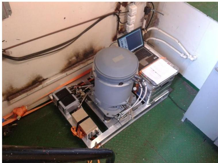
**Figure 2.4** Russian “Elektropribor” manufactured gravimeter Chekan-AM for marine gravimetric data acquisition, placed near the mass center of the vessel.
