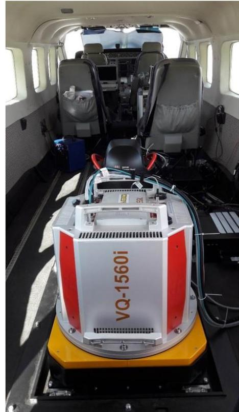
**Figure 4.6** RIEGL VQ-1560i LiDAR Scanning System (in the left figure) and it placed on the survey plane (in the right figure; survey plane in Figure 4.3) (Aerolaserskanner 2017b).
