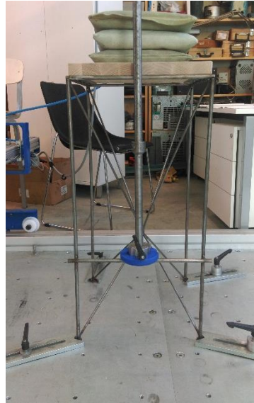
Figure 43. Foot rest static load test.
