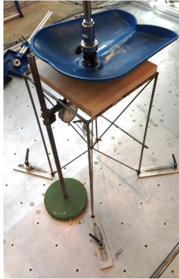
Figure 41. Seat static load test.
