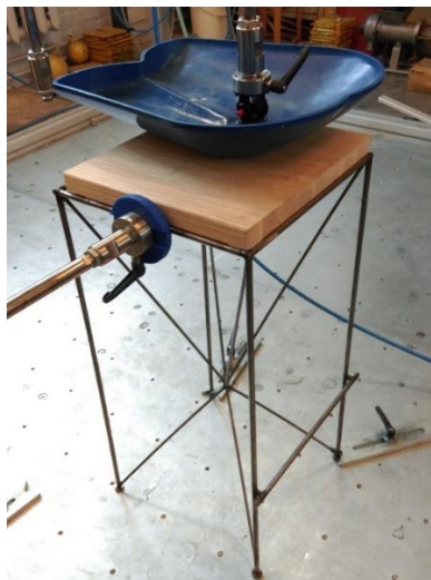
Figure 46. Leg sideways static load test.
