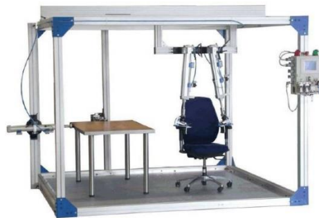
Figure 39. Universal test rig for alternating bending tests on furniture [44].
