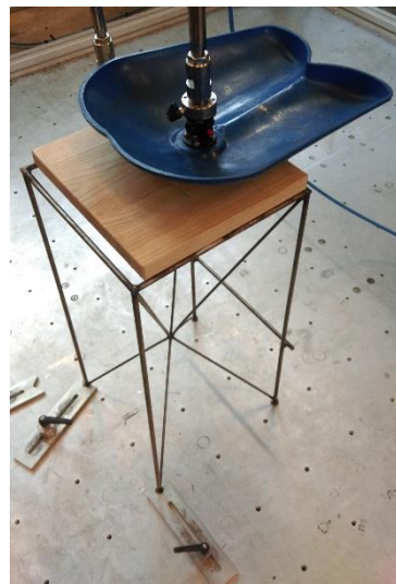
Figure 42. Seat front edge static load test.
