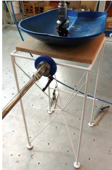
Figure 45. Leg forward static load test.
