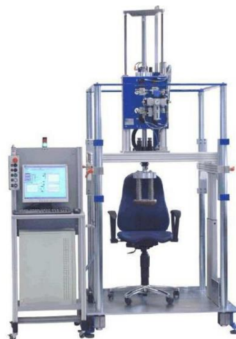
Figure 40. Drop test rig for impact loading of seating furniture [44].
