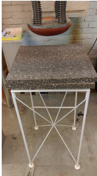
Figure 47. Seat impact test.
