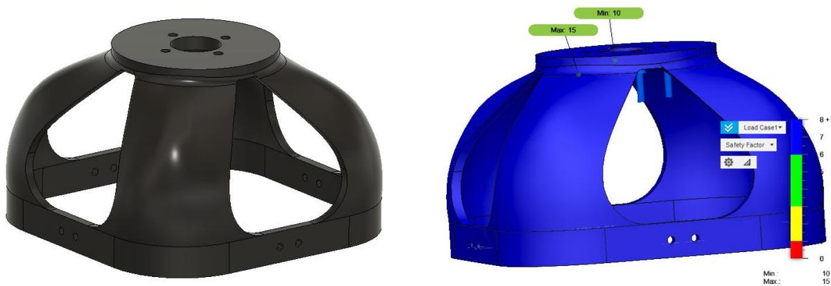
Figure 2.10. Upper Frame solid model and static stress simulation safety factor results.
