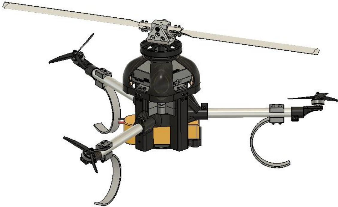
Figure 2.14. Experimental Y4 prototype – full CAD assembly
