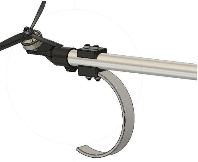
Figure 2.13. Landing gear PP-tube section and attachments
