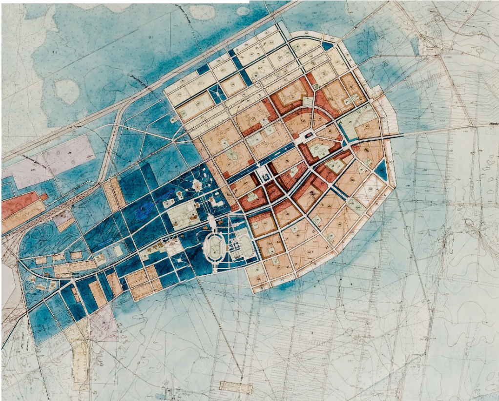
Figure XI. The main axes were crossing the centre of Kohtla-Järve, 1956, by design institute „Estongiprogorstroï” (Voldemar Toppel) following the version of Lengorstroyprojekt. In the middle: Victory Boulevard. At the bottom middle: stadium in the park. The park with pre-war settlement (on the left) formed the 2-kilometre sanitary zone (EAM 3.1.281)
