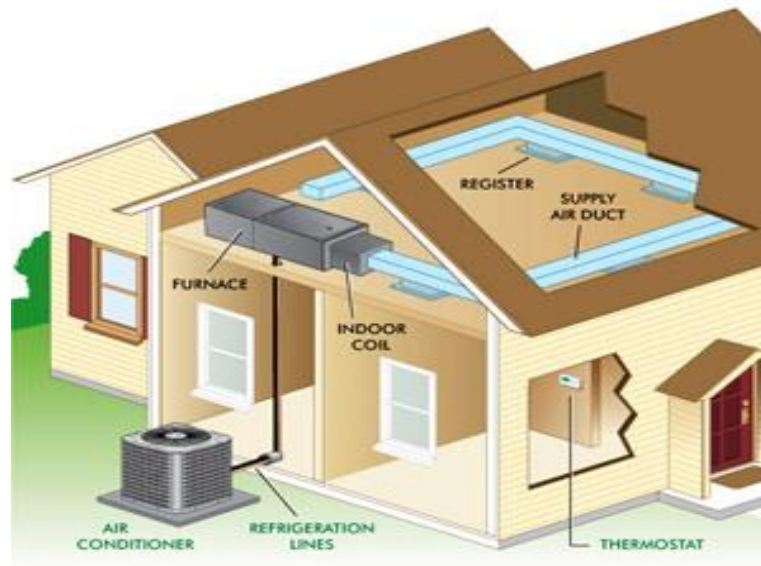
Figure 3.1. Diagram of Split HVAC System [17]
