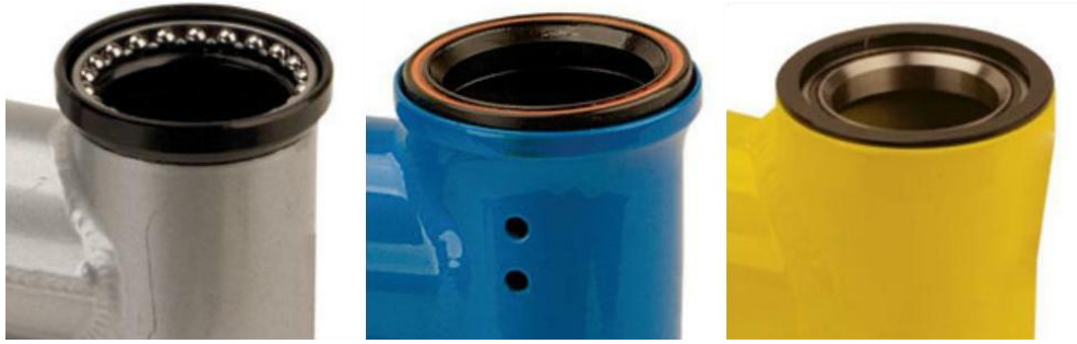
Figure 5.2. General headset types. Left - standard headset which has two bearing cups pressed into the headtube. Center - integrated headset have a proper taper machined into the headtube for bearing - therefore doesn't require a cup. Most of the chromoly frames have this concept. Right - internal headset requires a thin aluminium cup to be pressed into the frame. They are better than standard because it is very easy to install headset and easier to manufacture than internal headsets. Mostly used on aluminum race frames. [47]
