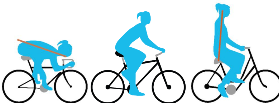
Figure 6.1. Bicycle geometry also defines sitting position on a bicycle. Left: road race position; center: semi-upright position; right: upright position
