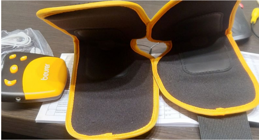
Figure 20. Beurer EM 29 device (left) and cuff with contacts (right).
