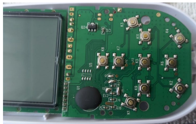
Figure 19. Sanitas SEM43 PCB front view.
