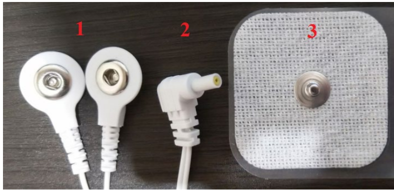
Figure 17. Sanitas cable connectors (1 – body connector side, 2 – device connector side) and body contact adhesive pad (3).
