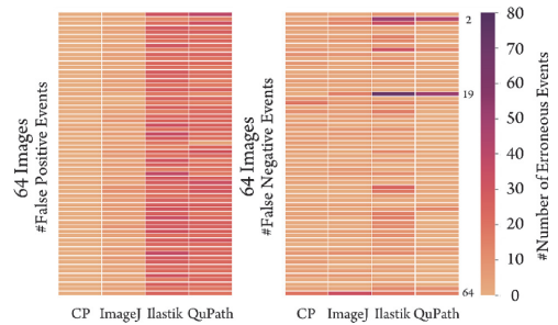
Figure 3. Droplet detection errors are higher in machine learning-based software in the diagnostic test. The figure shows the False Positive (FP, wrong detected droplet) and False Negative (FN, wrong undetected droplet) events per image. Each block represents event or image error detection. The scale shows the number of errors (dark = high and bright = low).
