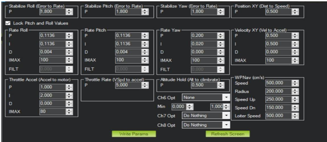
Figure 27. All quadcopter PIDs' values are set to maximum [25].
