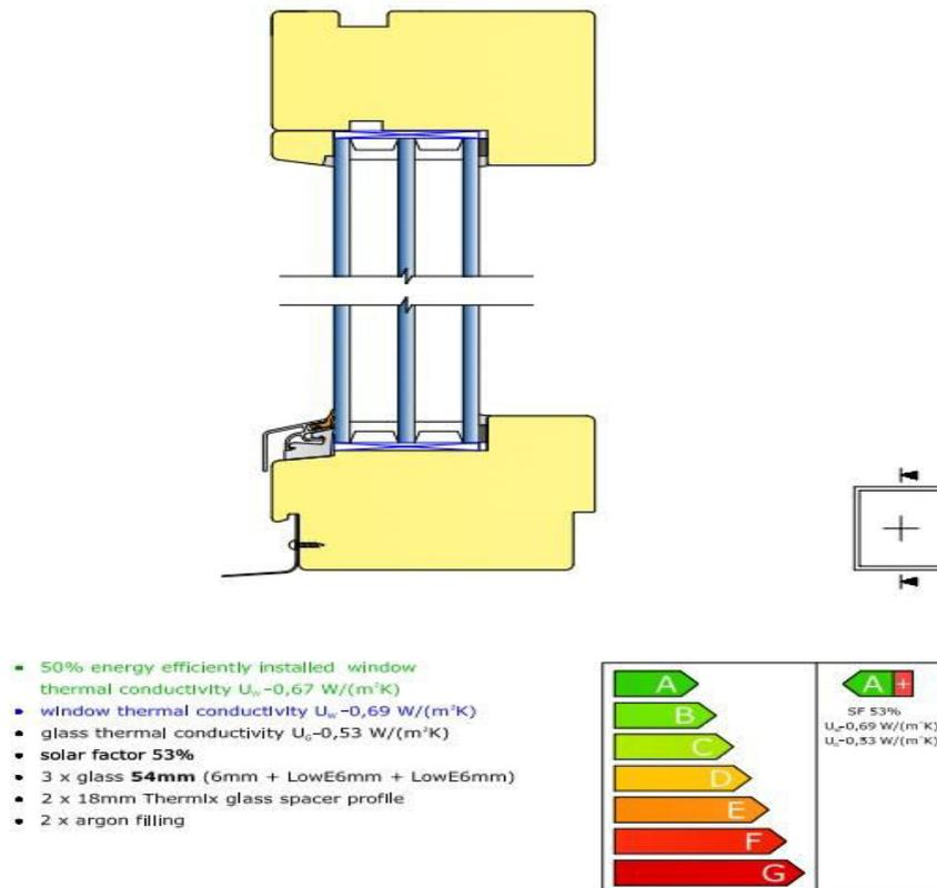
Figure4. A triple glazed, 2x18mm gap and 2x argon filled glass window
