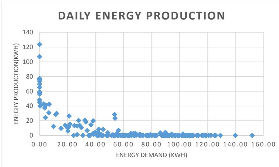
Figure 5. Daily energy production when the South windows of 375mm wall thickness building are halved.
