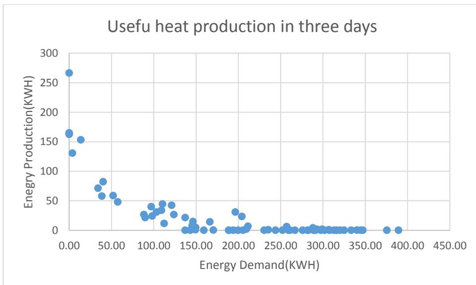
Figure 6. Energy production after three days for halved South windows
