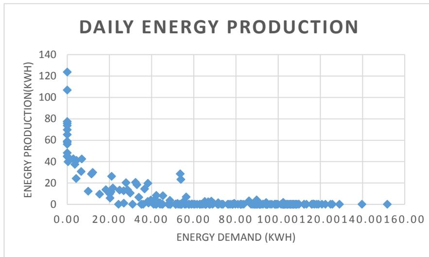
Figure6. The relationship between energy demand and production as shown by the slope indicates that the productivity of the system decreases at high energy demand
