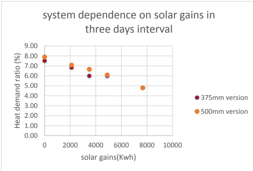
Figure 18. Linear decrease in heat demand ratio of the system with respect to increase in solar gains is higher after three days.
