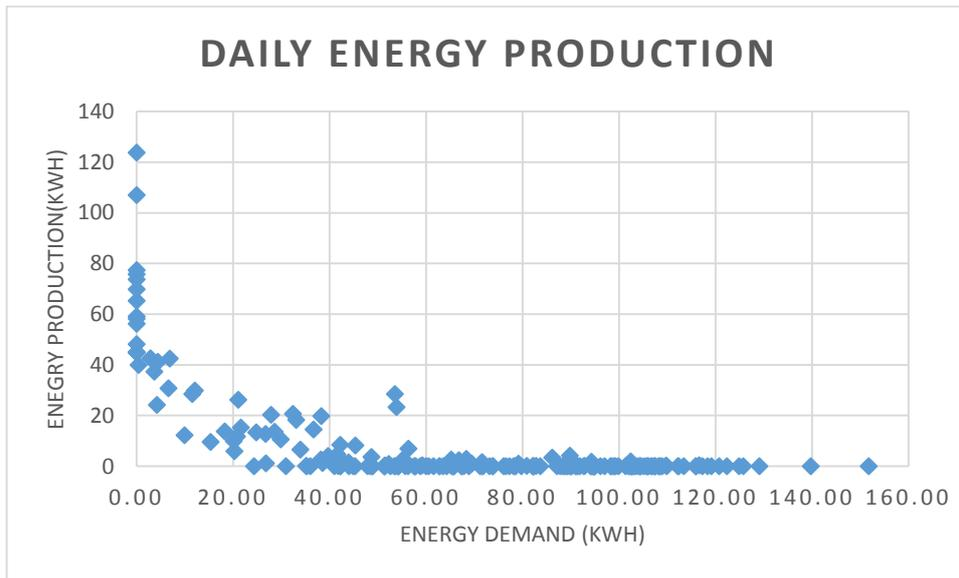
Figure9. Increase in energy production as a result of wall thickness modification to 375mm. The trend of energy production remains the same as in figure6 above that is as energy demand gets higher the slope of the curve starts to drop.
