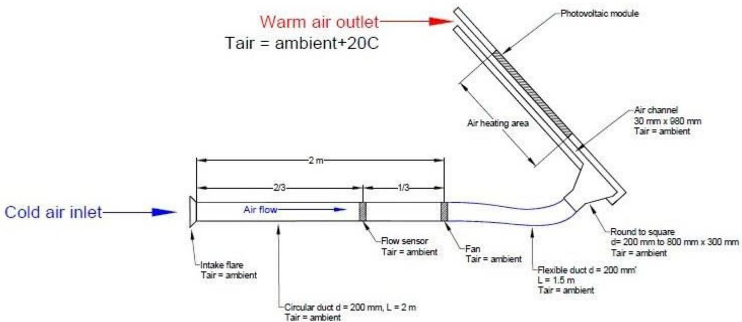
Figure 5. A 2m tube through which the inlet cold air enters the system to extract heat
