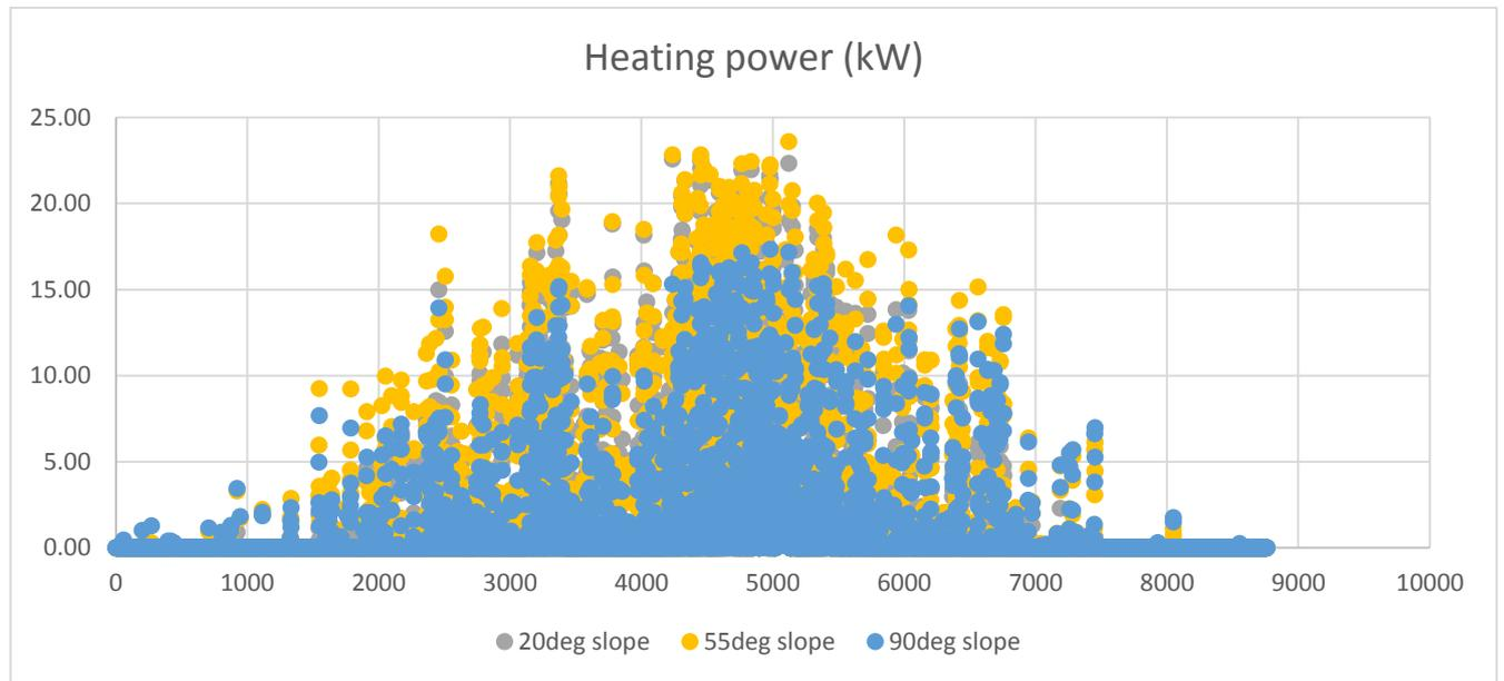
Figure8. Effect of change in angle of inclination on energy production with 55 degree indicating the best angle to be used (see yellow dots). Slope at angle 20degree shows poor power production ( grey dots).
