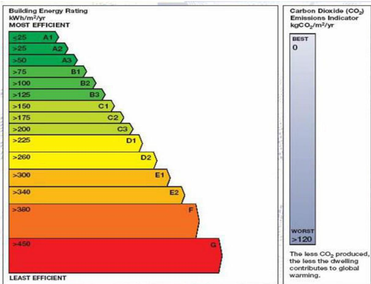
Figure 5: The building energy rating based on energy efficiency and carbon dioxide emission with Class A1 the most efficient and almost zero carbon dioxide and class G the least efficient
