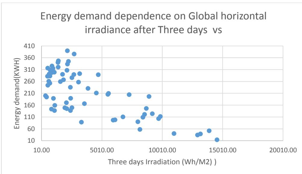
Figure 20. The decrease in Energy demand is high as global horizontal irradiance increases after three days.
