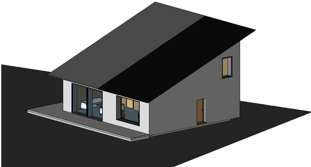
Figure1. 3D view of the simulated building with the black shading showing the 80m<sup>2</sup> surface area of the roof that is occupied by the PV panel.
