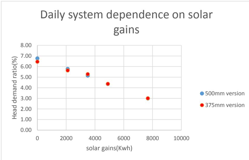
Figure17. Linear decrease in heat demand ratio of the system with respect to increase in solar gains.
