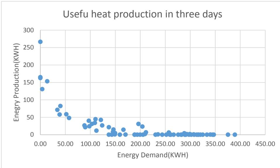
Figure 12. The energy production after three days increases from 628.17 (kWh) to 877.35 (kWh) when the south windows are halved
