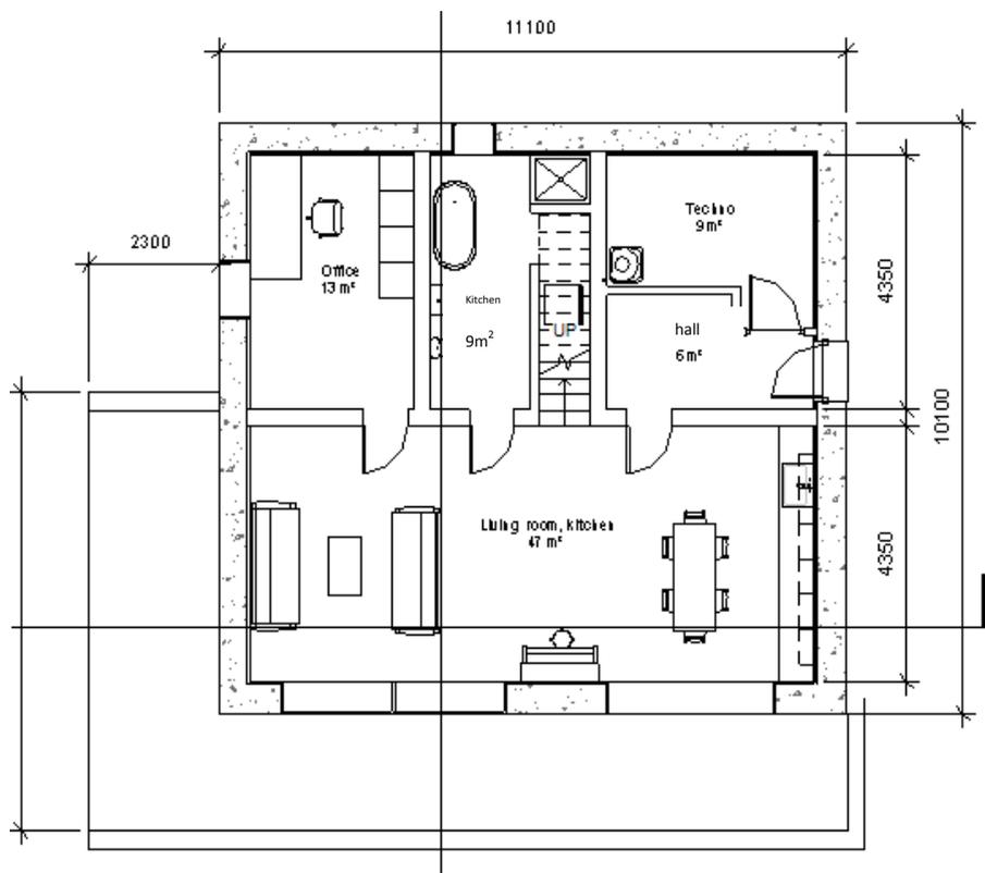
Figure2. Specific dimensions of the floor plan drawn between the walls specify room sizes
