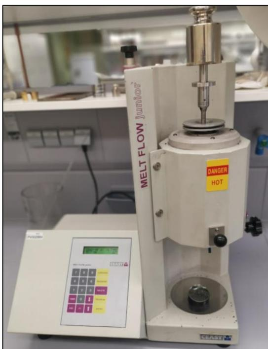
**Figure 6.** Melt Flow Tester
