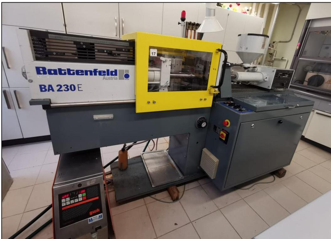
**Figure 3.** Injection molding machine Battenfeld BA230E
