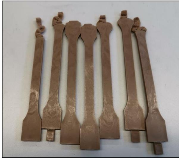
**Figure 4.** Appearance of short shots during injection moulding with an increment in ash content (before the optimization of process parameters)
