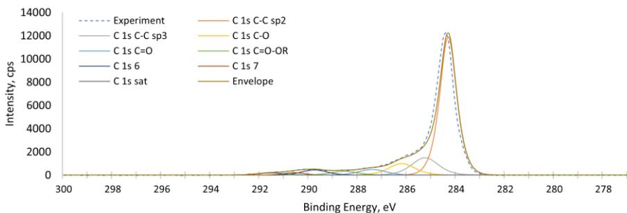
Figure 15. C 1s XPS fitting curve of CA-based SPME coating material.
