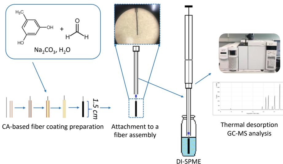
Figure 6. Schematic of the SPME CA-based fiber coating procedure, followed by DI-SPME-GC-MS analysis (**Publication III**).
