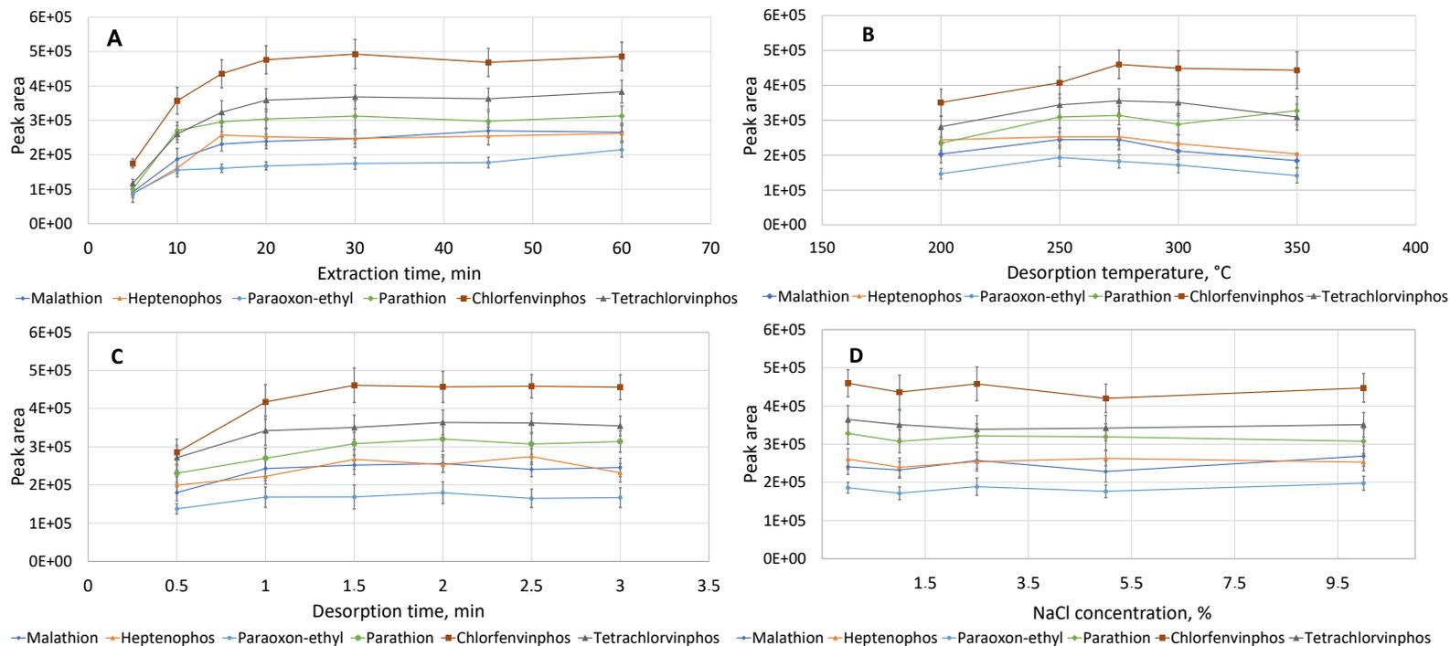
Figure 16. Effects of (A) extraction time, (B) desorption temperature, (C) desorption time, and (D) NaCl concentration on SPME efficiency. The concentrations in 0.5 mL of working solution include  $2.5 \text{ mg L}^{-1}$  heptenophos,  $2.7 \text{ mg L}^{-1}$  paraoxon-ethyl,  $3.7 \text{ mg L}^{-1}$  tetrachlorvinphos,  $2.6 \text{ mg L}^{-1}$  chlorfenvinphos,  $2.9 \text{ mg L}^{-1}$  parathion and  $3.3 \text{ mg L}^{-1}$  malathion (**Publication III**).
