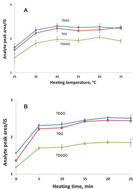
**Figure 2.** Effect of heating temperature (A) and time (B) on derivatization efficiency.
