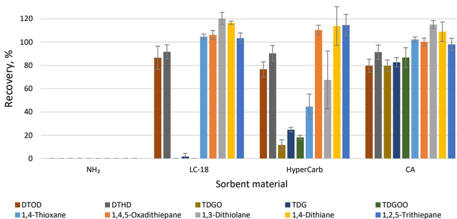
Figure 11. Comparison of the performances of CA-based and commercially available sorbents for the SPE of HD degradation products under optimised conditions (**Publication II**).
