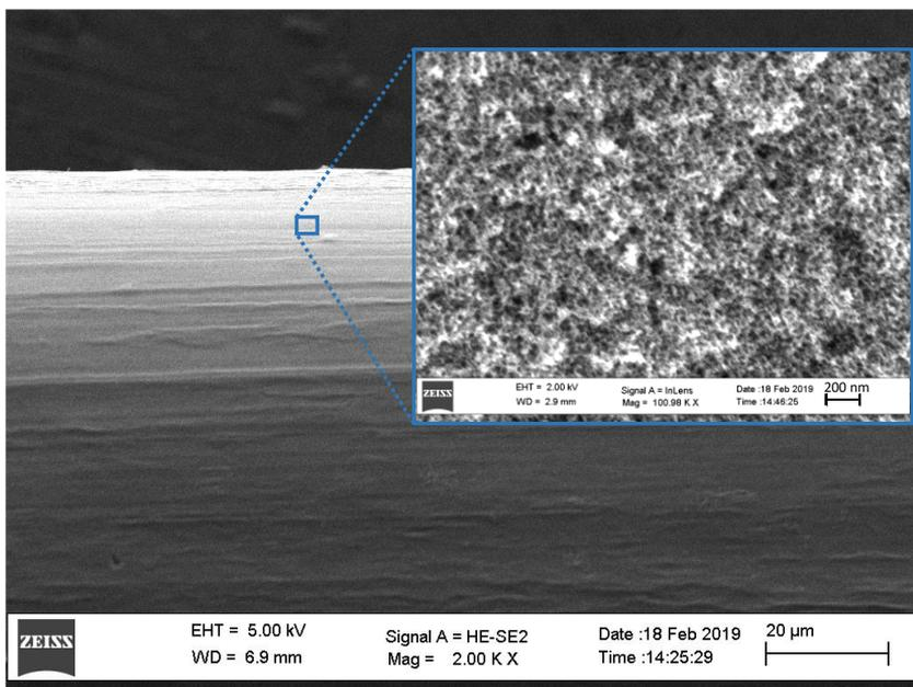
Figure 13. SEM image of the CA-coated SPME fiber surface.
