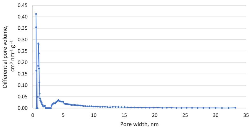
Figure 14. Pore-size distribution of CA-based SPME coating material.
