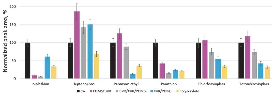
Fig. 4 Extraction of OPPs from water samples using different SPME fibers.
