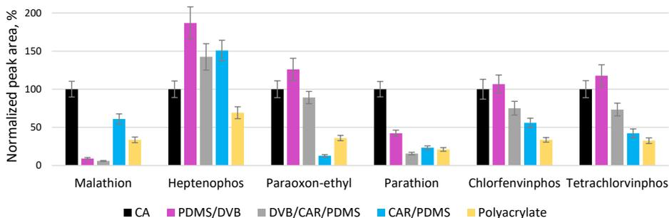
Figure 19. Extraction of OPPs from water samples using different SPME fibers (**Publication III**).
