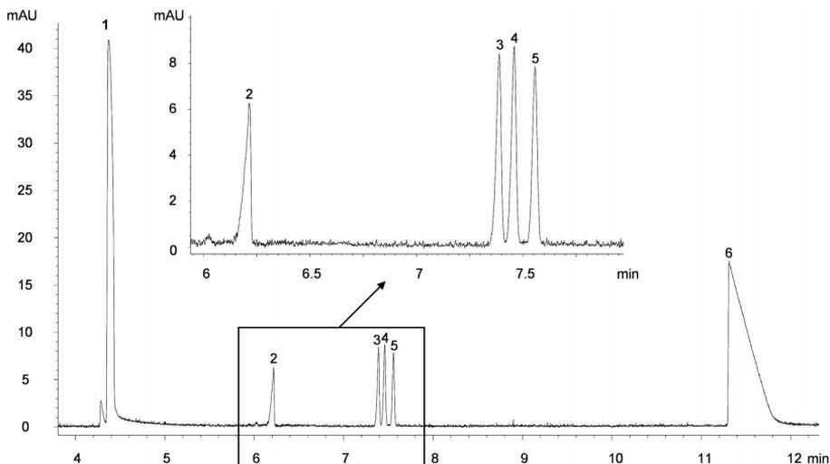
**Figure 3.** Representative electropherograms obtained after derivatization of 3.05  $\mu\text{g/mL}$  of TDG (4), 3.45  $\mu\text{g/mL}$  of TDGO (3), and 3.85  $\mu\text{g/mL}$  of TDGOO (5) under optimized separation conditions: borate buffer concentration 30 mM, buffer pH 8.5, applied voltage 15 kV, and capillary temperature 25°C. Additional peaks: EOF (1), IS (2), and phthalic acid (6).
