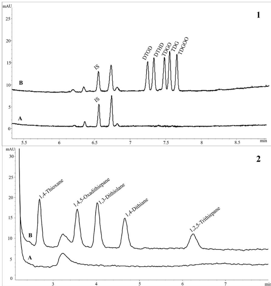
Fig. 4. Electropherograms (1) and chromatograms (2) obtained after applied all the sample pretreatment steps and HPLC/CE-DAD analysis: A) 10 mL pore water sample from the Bornholm Deep; B) 10 mL pore water sample from the Bornholm Deep spiked with aliphatic and cyclic HD degradation products at final concentrations of 10 and 5  $\mu$ M, respectively (50  $\mu$ M of IS for CE-DAD analysis).
