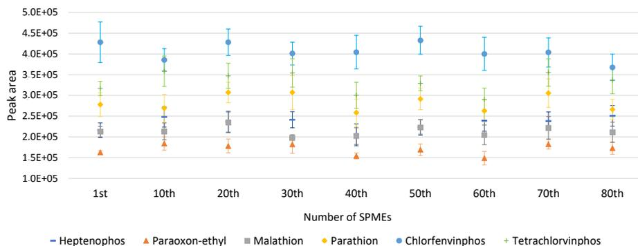
Figure 18. Reusability of CA-coated SPME fiber. The concentrations in 0.5 mL of working solution include 2.5 mg L<sup>-1</sup> heptenophos, 2.7 mg L<sup>-1</sup> paraoxon-ethyl, 3.7 mg L<sup>-1</sup> tetrachlorvinphos, 2.6 mg L<sup>-1</sup> chlorfenvinphos, 2.9 mg L<sup>-1</sup> parathion, and 3.3 mg L<sup>-1</sup> malathion.
