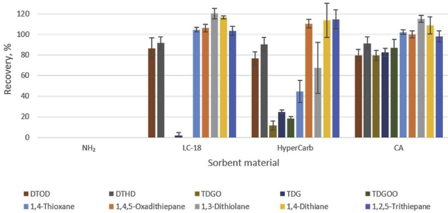
Fig. 3. Comparison of the performances of CA-based and commercially available sorbents for the SPE of HD degradation products under optimized conditions.
