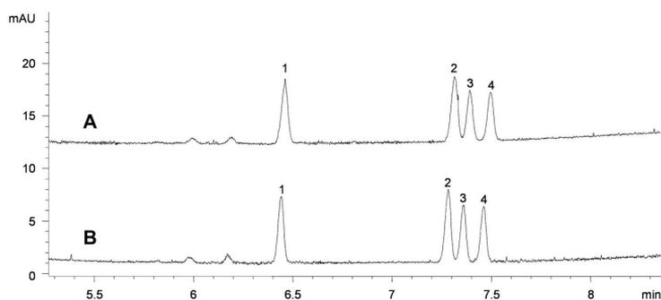
**Figure 4.** Electropherograms of (A) distilled water and (B) seawater samples. Separation conditions: borate buffer concentration 30 mM, buffer pH 8.5, applied voltage 15 kV, and capillary temperature 25°C. Peaks: IS (1), TDGO (2), TDG (3), TDGOO (4).
