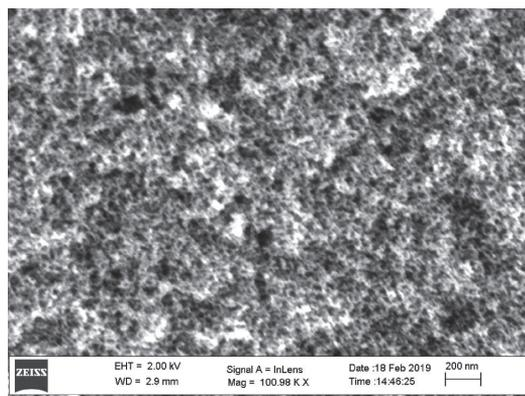
Fig. 1 SEM image of the surface of the CA-coated SPME fiber.
