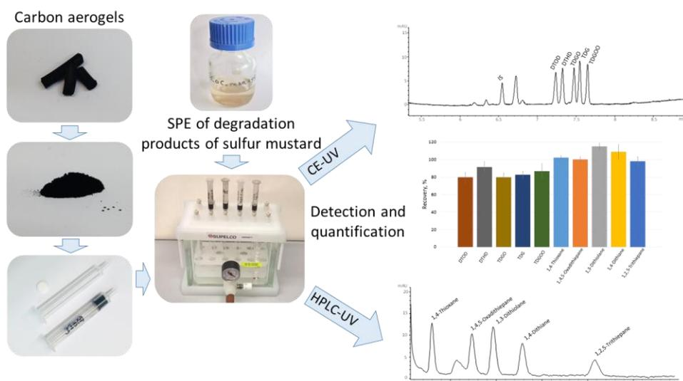
Figure 5. Schematic of CA-based SPE cartridge preparation followed by SPE-CE/HPLC-UV analysis (Publication II).
