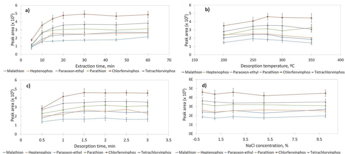
Fig. 2 The effect of different factors on SPME efficiency. (a) Extraction time, (b) desorption temperature, (c) desorption time, (d) NaCl concentration. The concentration of OPPs in 0.5 mL of working solution, 2.5 mg L<sup>-1</sup> heptenophos, 2.7 mg L<sup>-1</sup> paraoxon-ethyl, 3.7 mg L<sup>-1</sup> tetrachlorvinphos, 2.6 mg L<sup>-1</sup> chlorfenvinphos, 2.9 mg L<sup>-1</sup> parathion and 3.3 mg L<sup>-1</sup> malathion.
