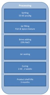
Figure 1 – Production scheme of spice-cured sprats "Sprats of Tallinn".
