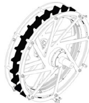
Fig. 1. Constructional schematic of the designed generator.
