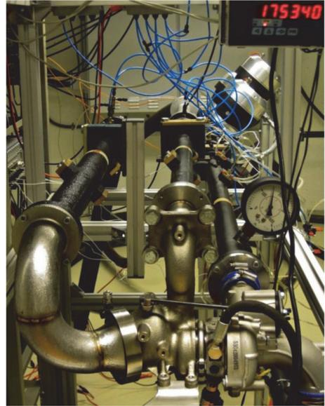
Figure 1. A photo of the test-rig in the facility for turbocharger acoustic measurements at CCGEx.
