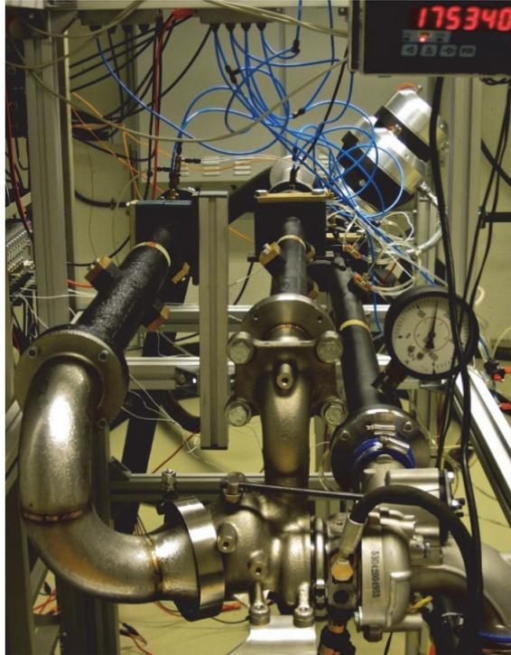
*Figure 1.2. A photo of the test-rig in the facility for turbocharger acoustic measurements of the CCGEx.*
