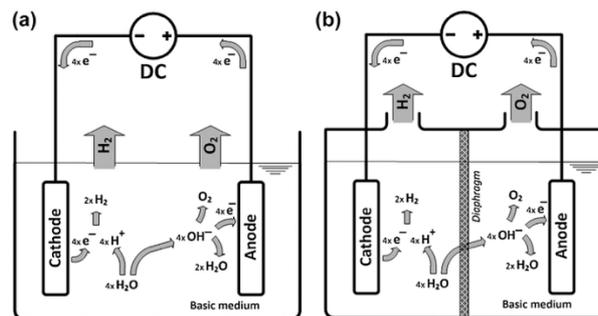
Figure 8. (a) Basic principle of an open EL cell in basic medium. Stoichiometric factors are related to the generation of one molecule of oxygen. As the half-cells are open oxyhydrogen is produced. (b) Deploying a semipermeable diaphragm between the two half-cells allows the separation of the two gases. [11]
