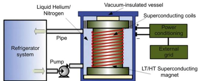
Figure 7. Schematic of distributed SMES system [16]
