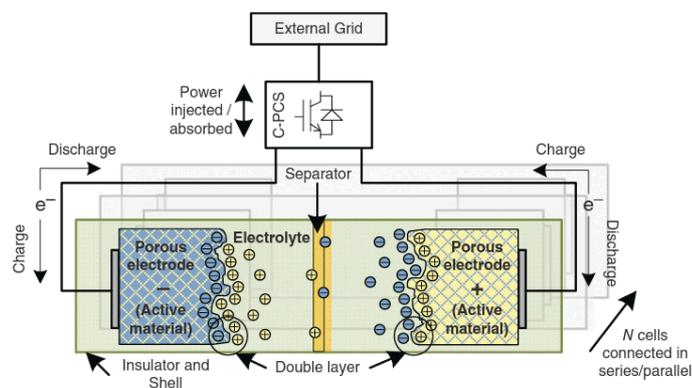
Figure 6. The illustrative topology of a supercapacitor, depicting the electrical double layers at each electrode/electrolyte interface [13]
