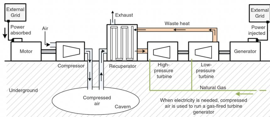
Figure 4. The operating principle of compressed air energy storage (CAES). [13]
