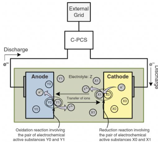
Figure 10. The operating principle of battery
