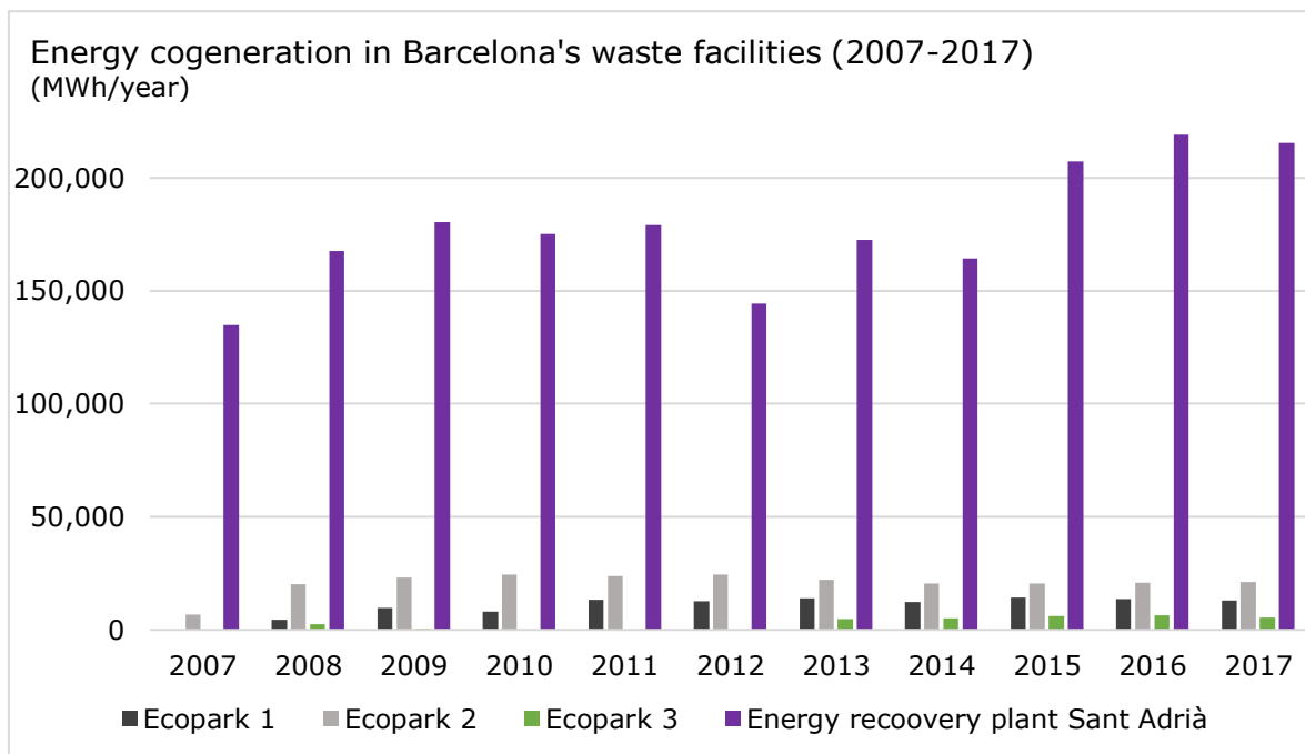
Figure 2.6 Energy generation through cogeneration processes in waste facilities in Barcelona (2007-2017) (Metropolitan Area of Barcelona, 2018).
