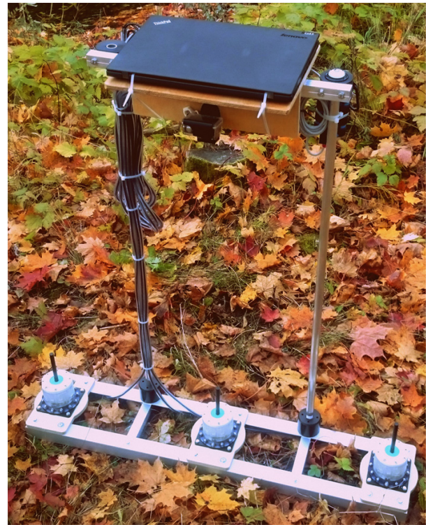
Fig. 1. (Left) Pressure-inertial hydromast breakdown. (Right) Field setup with triple hydromast array.
