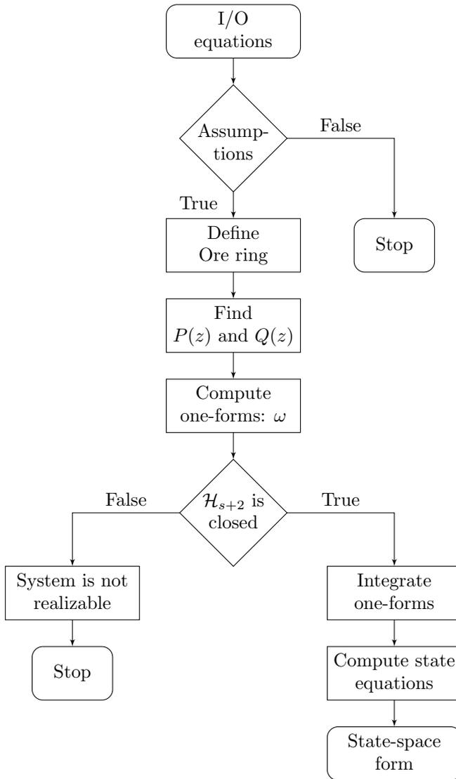
Figure 6.1: The block-diagram of the function Realization
