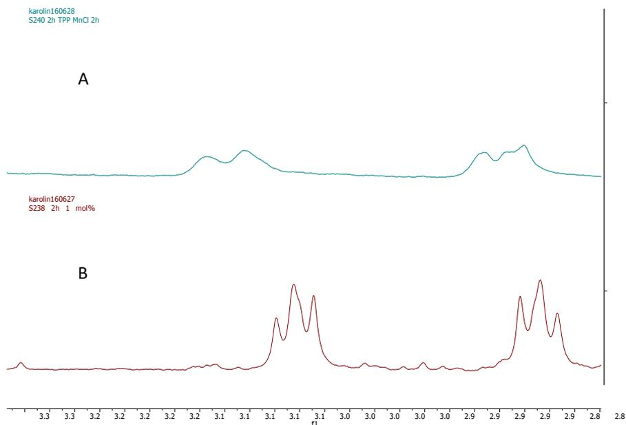
Figure 9.  $^1\text{H}$  NMR shifts of diacid (A) and diketoacid (B).
