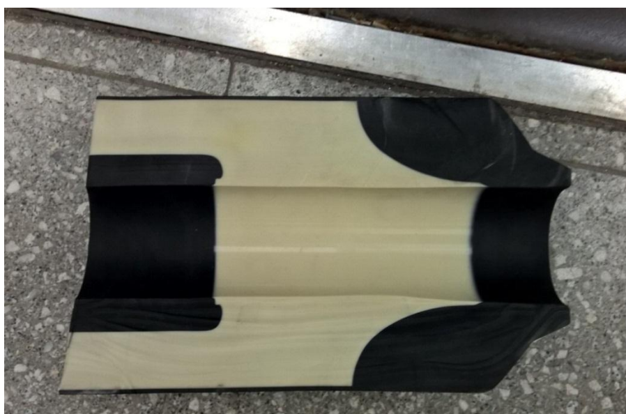
Figure 1.7. Stress cone in joint insulation.
