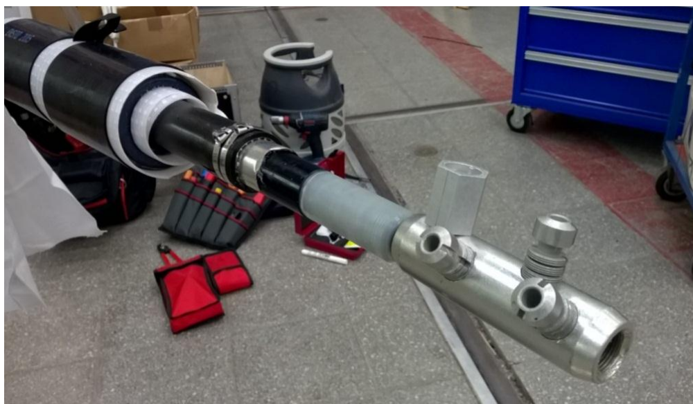
Figure 4.2. Aluminium connector for connecting the conductors.
