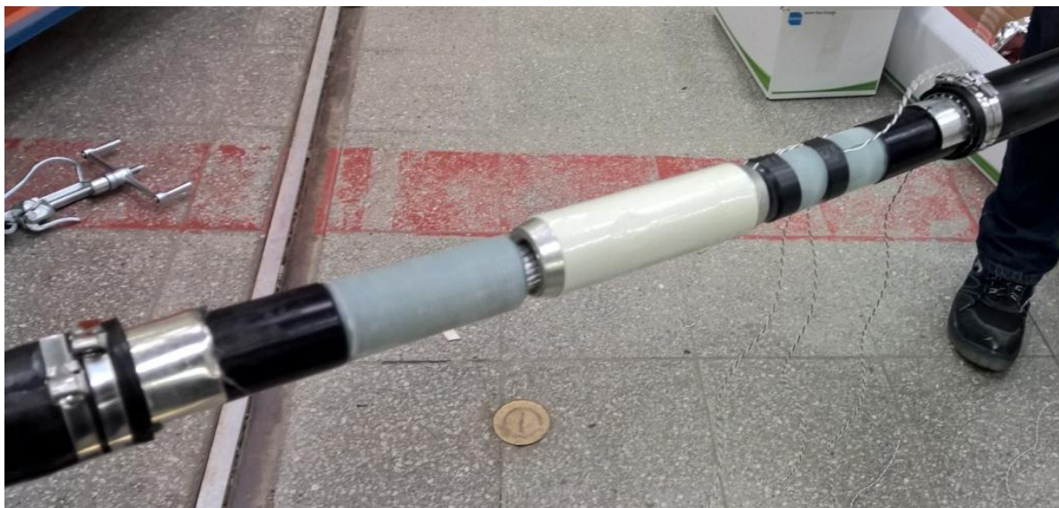
Figure 4.3. The unfinished joint with some thermocouples visible.
