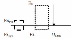
Figure 6.3 Dependent link tolerance (Es and Ei) and uncertainty of systematic factors (index sys)
