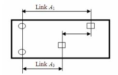
Figure 6.5 Dimensional chain for the elementary control set of mobile phone circuit boards.
