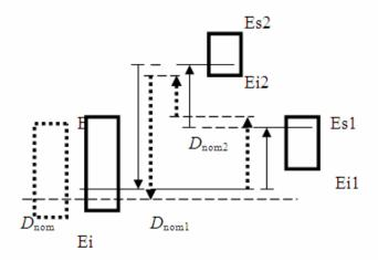
Figure 6.2 Dimensional chain movement (shift) caused by systematic factors
