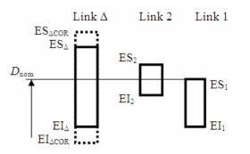
Figure 6.6 Movement of dimensional chain links through the influence of factors:
