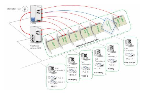
Figure 3.3 KLMS and simplified process flow
