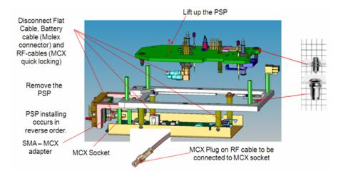
Figure 4.7 Implemented technical solution (Patent No.: FI119529B1)
