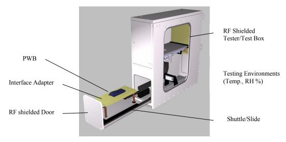
Figure 5.3 PWB Level Tester for manual and semi-automated test
