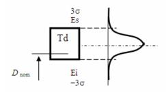
Figure 6.1 Tolerance structure allowing the use of normal distribution statistics
