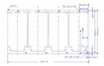
Figure 5.6 Placement and main parameters of test points on the test plate in PWB panel (PWB contour only for illustrative example)
