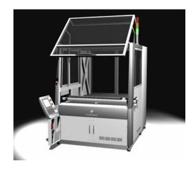
Figure 4.2 Example: Unified standard frame module (JOT Automation)
