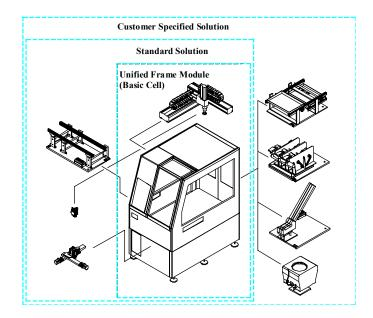
Figure 4.1 Unified basic robot cell and unified modules concept
