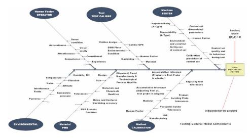
Figure 5.7 Mechanical Test System General Model - Inputs Tree
