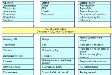
Figure 5.8 Circuit boards testing general model - Uncertainty Tree
