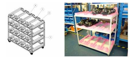
Figure 2.10 Multifunctional modular storage rack: model and rack in use
