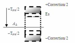
Figure 6.4 Dependent link summary tolerance scheme including systematic factor uncertainty and corrections if those can't be exactly estimated
