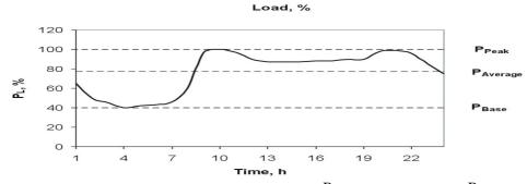
Figure 3.2 A typical daily power system load curve:  $P_{Base}$  - daily basic load,  $P_{Peak}$  - peak load,  $P_{Average}$  - average load.
