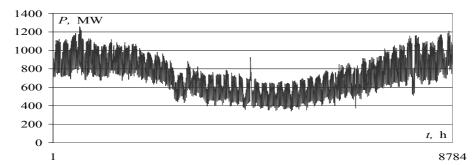
Figure 3.4 Example of a yearly power system load diagram
