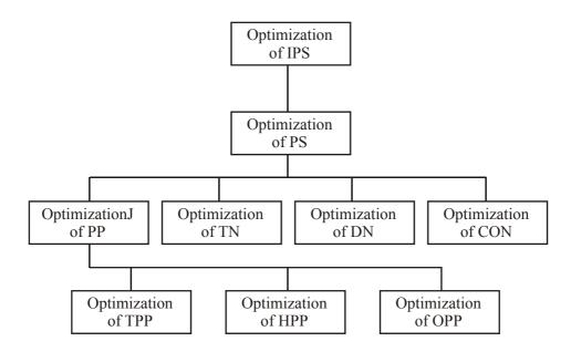
IPS – interconnected power system, PS – power system, PP – power plants, TN – transmission network, DN – distribution network, CON – consumers, TPP – thermal power plants, HPP – hydroelectric power plants, OPP – other power plants
