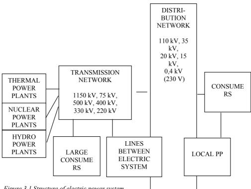
Figure 3.1 Structure of electric power system
