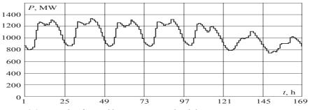
Figure 3.3 Example of a weekly power system load diagram
