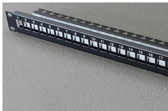
Figure [39] 19-inch RJ45 panel
