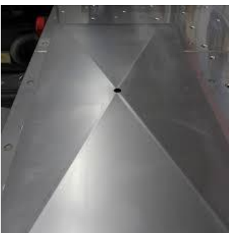
Figure[81] Diagonal ribs
