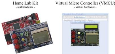
Fig. 8 – Robotic HomeLab kit and VMCU
