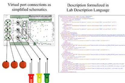
Fig 3. - Description of virtual port connection in LDL
