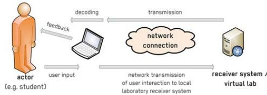
**Fig. 2.** A virtual or simulation laboratory
