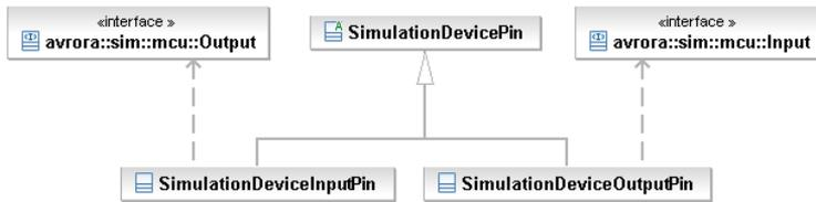
**Figure 4.4.:** Virtual pins of hardware module
