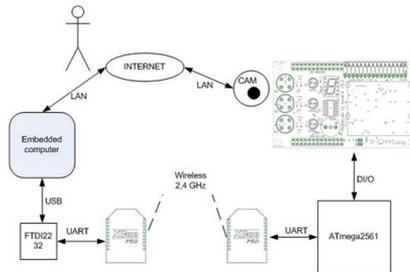
Fig. 9 – VMCU platform with user interface module
