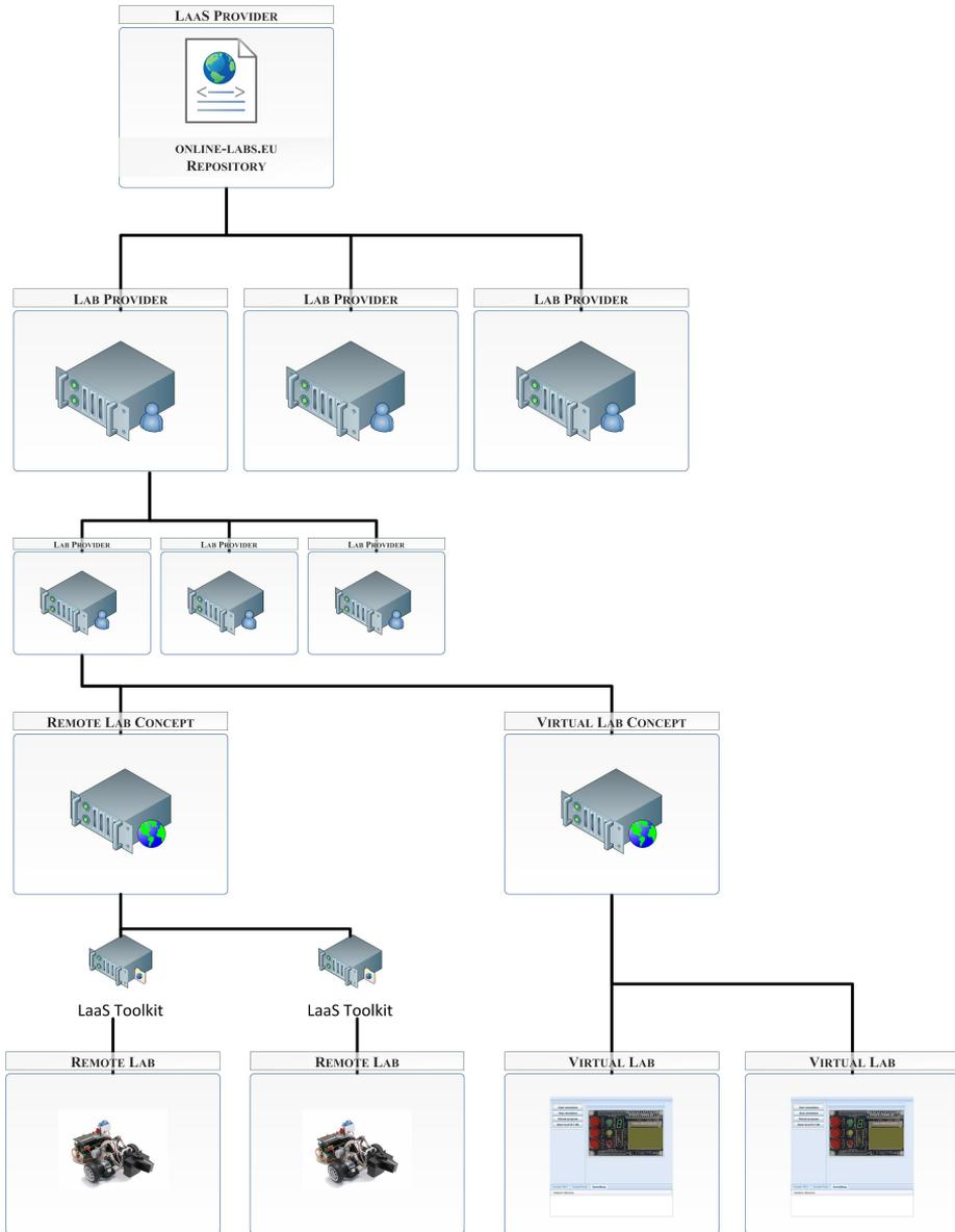
Figure 3.2.: LaaS System structure from a technical point of view
