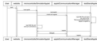
Fig. 6 – Sequence diagram of Communication manager
