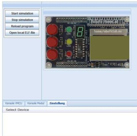
Fig. 5. Overview of Virtual MCU device and User Interface module
