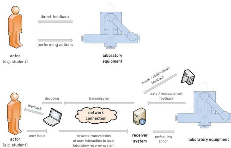
Fig. 1. A common vs. a remote laboratory
