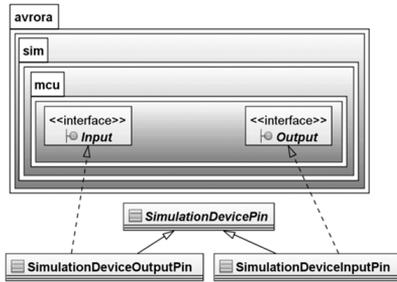
Fig. 5 – Virtualized I/O concept
