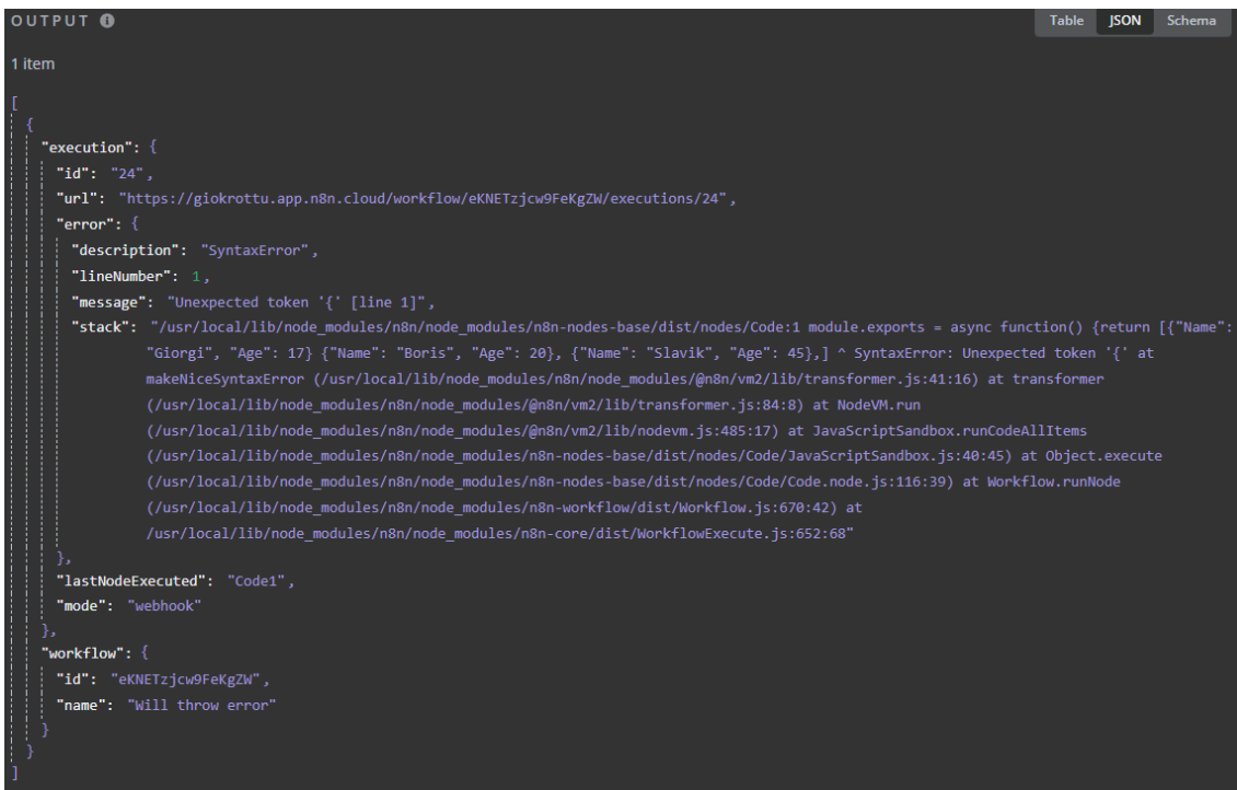
Figure 15: N8n – a syntax error caught by a workflow with the “Error Trigger”
