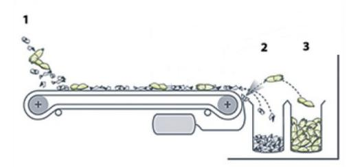
Figure 6. Schematic model of simple automated single line segregator. Where: 1 – waste income, 2 – container for heavy waste, 3 – for light-weight waste
