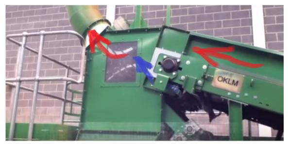
Figure 20. High-velocity air flow separation module. White paper moves shown with red. Air jets shown with blue.
