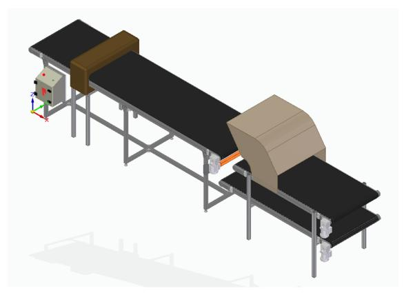
Figure 26. Conveyor line assembly. 3D model.
