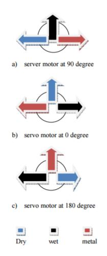
Figure 10. Rotation of circular base of servo [7]
