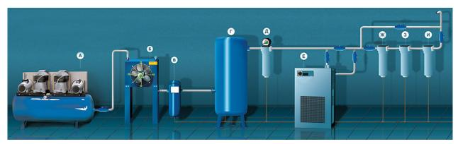
Figure 23. Pneumatic system air preparation module, in which (form left to right: Compressor; air cooler; cyclone type separator; reservoir; preliminary filter; air drier; intermediate with condensate remover; oil catching filter; coal filter) [13].
