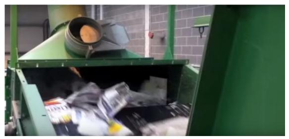
Figure 19. Paper separation with air jet
