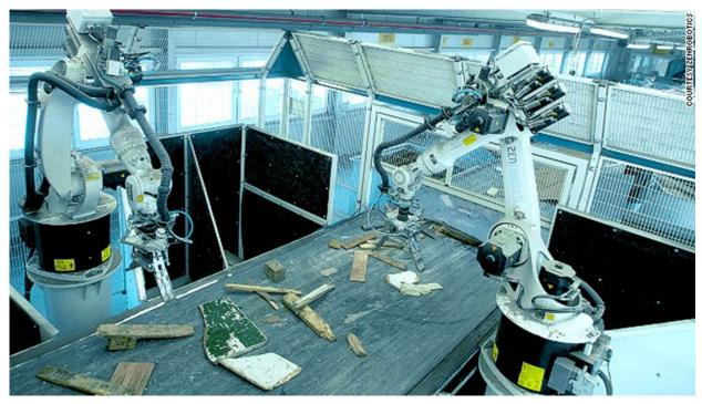
Figure 15. Alternative solution for manipulator segregation module on rotary axes
