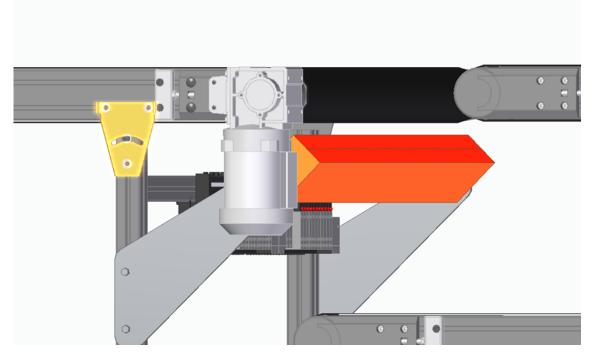
Figure 22. 3D model of separation module. On the right there are two conveyor lines, upper for separated white paper, and lower for other materials. The nozzle block is in the middle right under the end of first conveyor.
