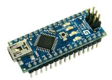
Figure 11. Arduino Nano microcontroller
