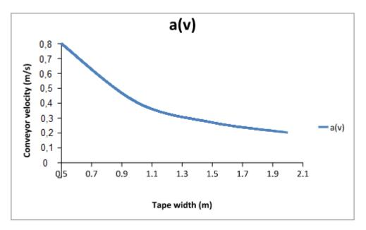
Figure 27. Tape width and velocity dependence
