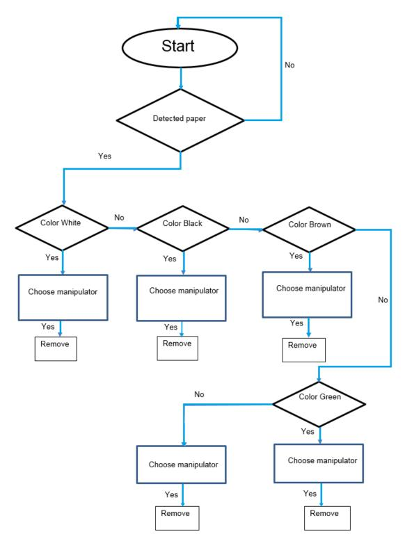
Figure 18. Control software logic chain
