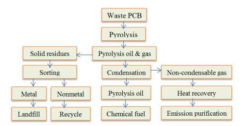
Figure 24, Pyrolysis method of electronic remanufacturing
