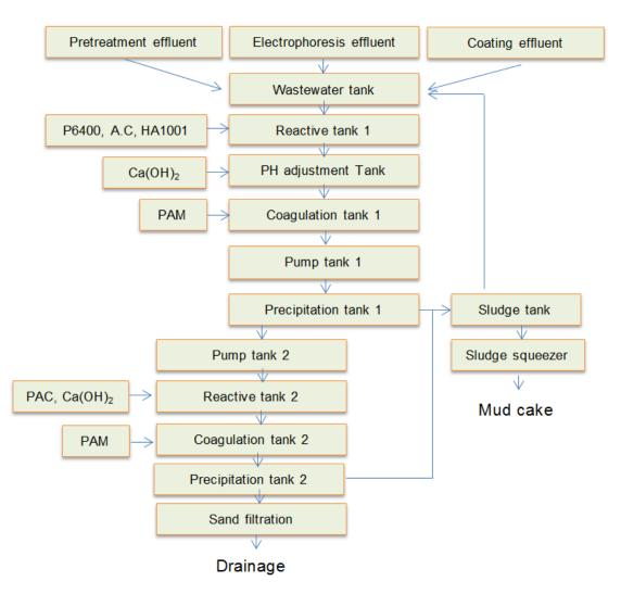
Figure 12, Green circulation processing flow of Coating Effluent [18] [26]
