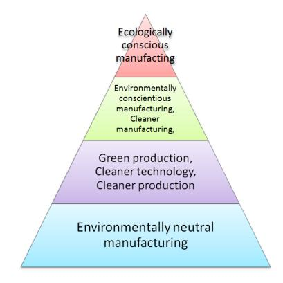
Figure 2, the four layers of the Green in manufacturing [2]
