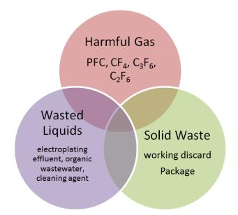
Figure 20, Three mainly wastes in the manufacturing of electron components
