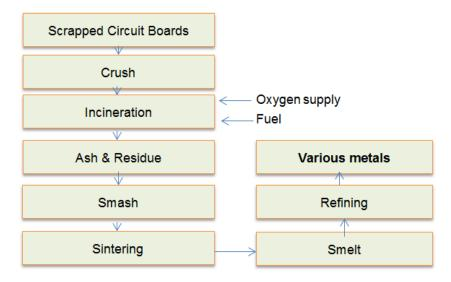
Figure 23, Incineration method of electronic remanufacturing
