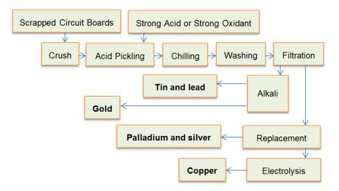
Figure 22, Chemical approach process of electronics remanufacturing
