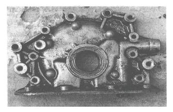
Figure 17, Engine cover after burning [27]
