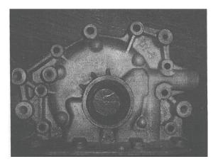
Figure 18, Engine cover after blast cleaning [27]
