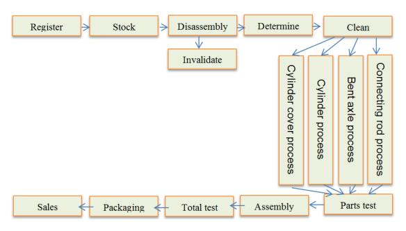
Figure 15, Process flow of engine remanufacturing [27]
