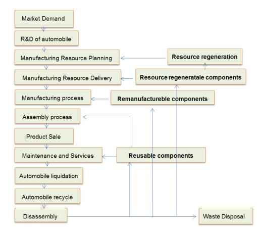
Figure 7, Product life cycle of automobile Green Manufacturing [26]
