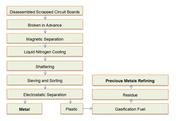
Figure 21, Process Routing of Physical Method
