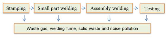
Figure 10, Process and problem of welding [18] [26]
