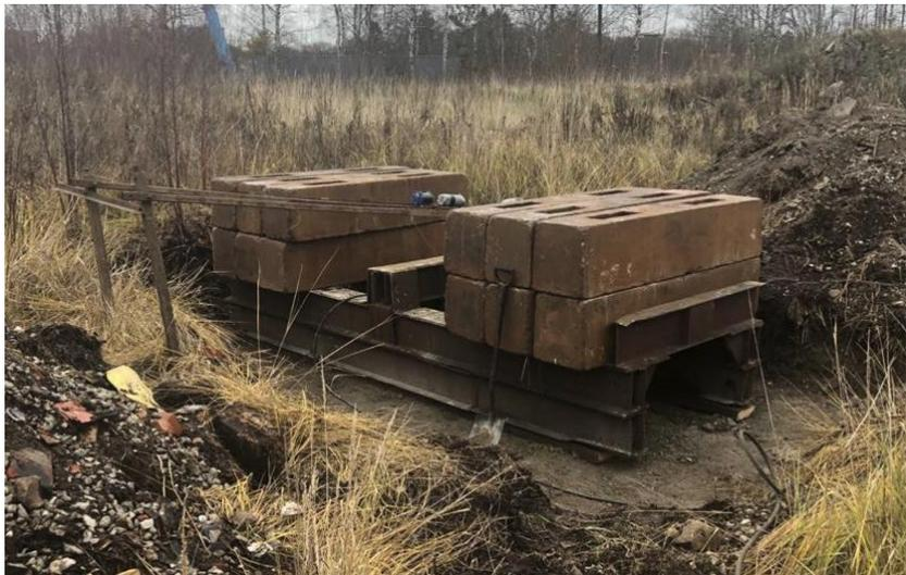
**Figure 18.** Scheme of a static pile load test.
