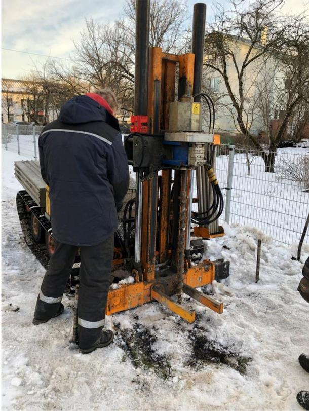
**Figure 20.** Lightweight truck equipped with a pre-drilling nozzle.
