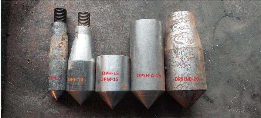
**Figure 25.** A selection of dynamic probing cones.
