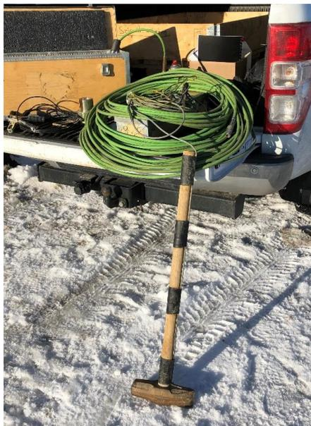
**Figure 31.** Sledgehammer connected to cable.
