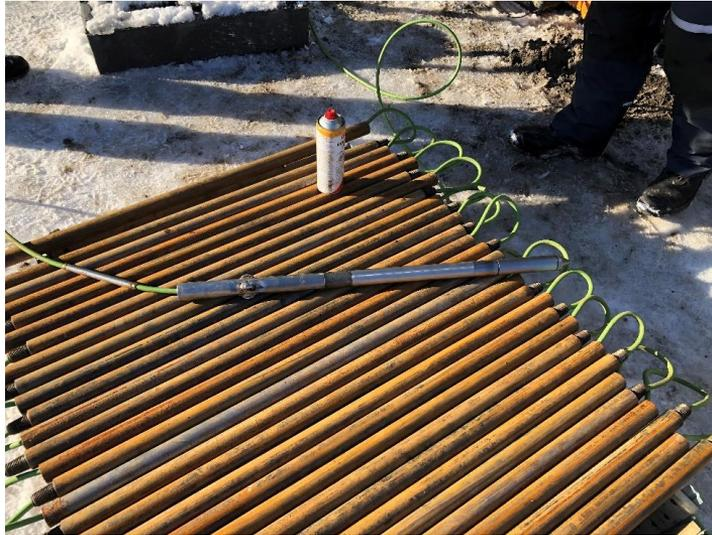
**Figure 30.** On top of the sounding rods is a CPTu probe connected to the seismic module and cable.
