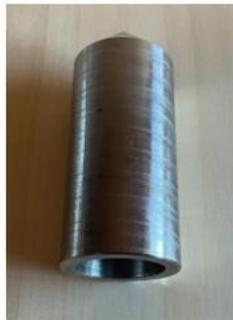
**Figure 27.** SDT penetrometer cone.
