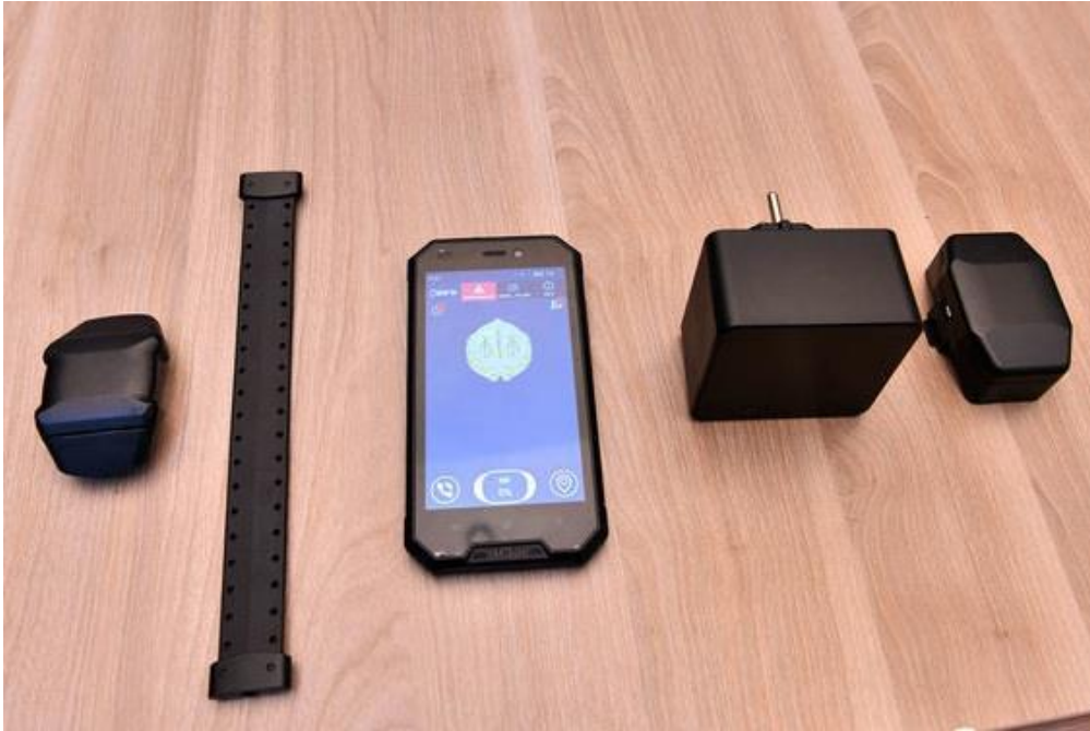
Figure 5. Surveillance equipment consists of Smartphone, bracelet and charging device
