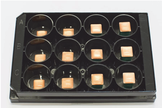
Figure S1. Set-up of 12-well microplate for optimal signal collection from bioluminescent bacteria on 1×1 cm copper surfaces. Photograph of a 12-well microplate in which the left column represents copper coupons on the plate bottom; left and right middle columns show coupons raised using 5 and 12 mm adapters, respectively; and the right column shows adapters raised using 15 mm plastic adapters; 75 \mu L bacterial suspension was applied to each copper coupon.
