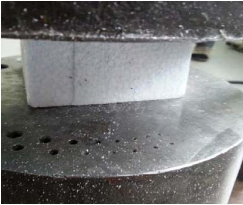
Figure 19. EPS120 ready to be impacted
