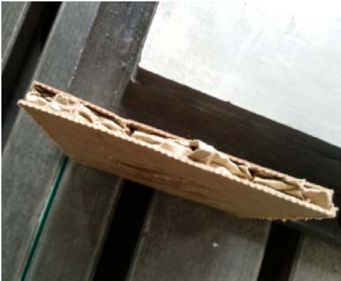
Figure 23. Honeycomb after the impact
