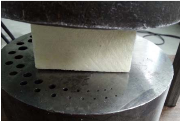
Figure 20. EPS50 ready to be impacted
