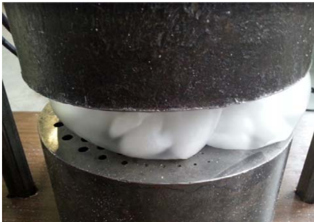
Figure 18. EPS granules ready to be impacted
