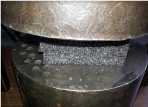
Figure 22. EPE ready to be impacted
