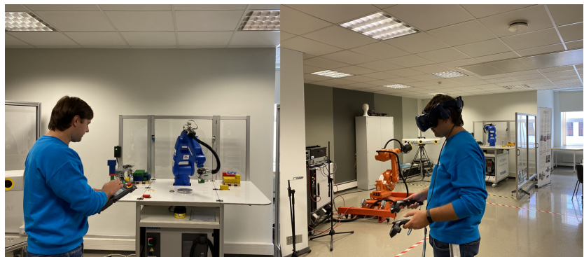
Figure 1. The design of experiments utilizes both physical and virtual representations of the work cell. The physical trials (left) involve the operator using the robot’s teach pendant to manipulate the end-of-arm tooling. The virtual trials use a VR interface (right) for commanding robot motions.
