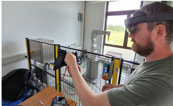
Figure 7: The AR setup with ABB1200 robot. The operator is manipulating the augmented path planning tool.
