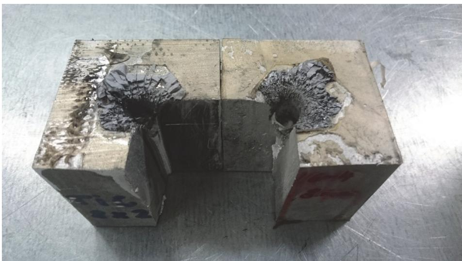
*Figure 3.15. Comparison of the mode of fragmentation between TiC-NiMo tile on the left and SiC tile on the right*
