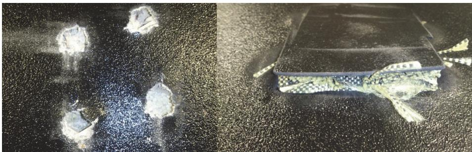
Figure 3.11. Certified armour panel according to NATO STANAG 4569 level 3 (WC core) after test firing according to AEP-55: a) front side; b) back side
