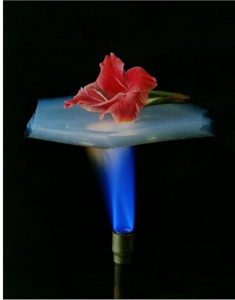
Figure 9. Silica aerogel protects flower from heat of Bunsen burner (Condliffe, 2014)
