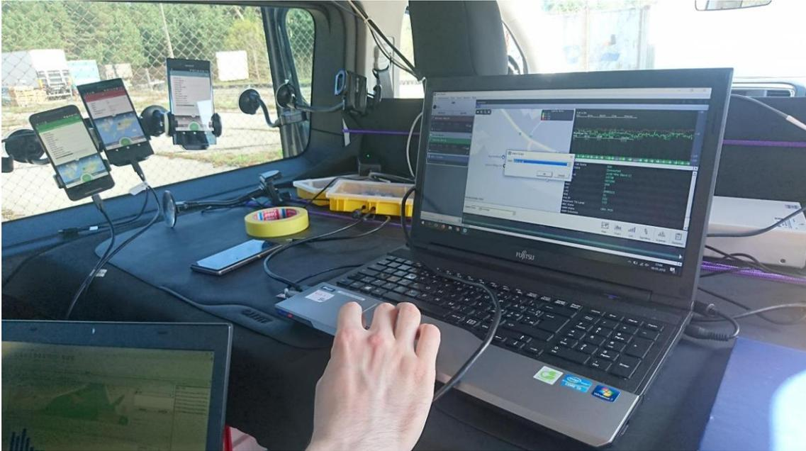
Figure 6. Placement of the mobile phones on window and USB hub (inside yellow box).
