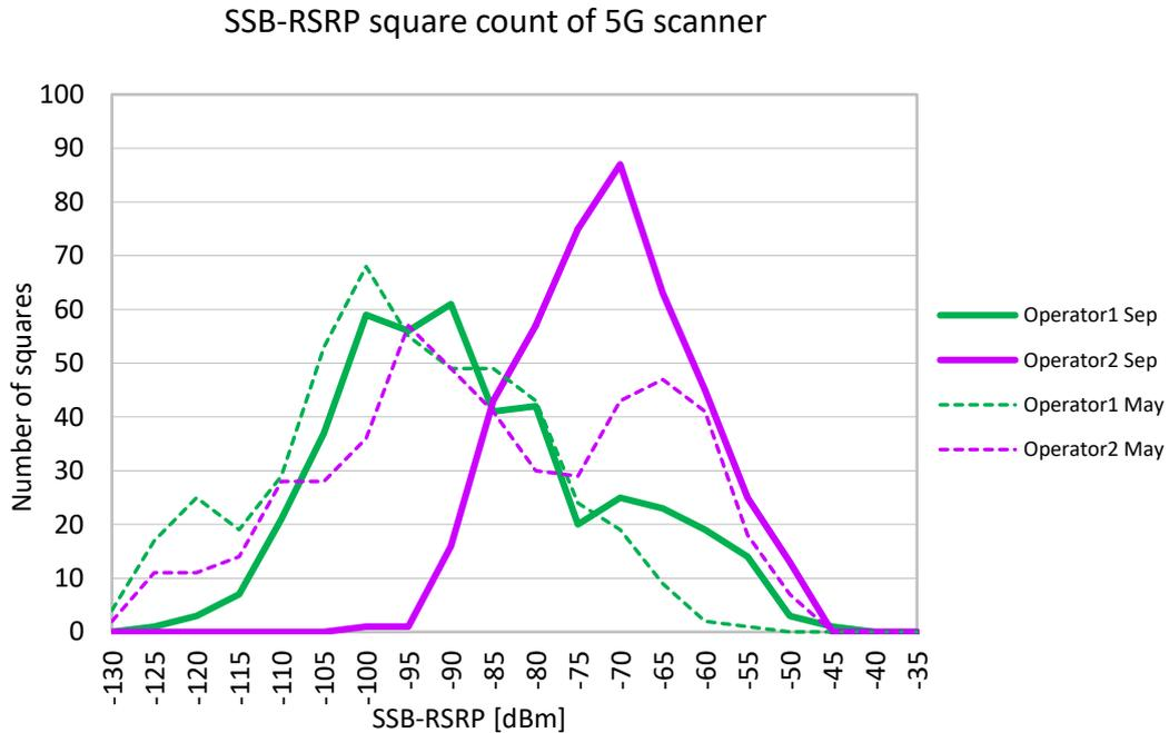
Figure 14. Square count of scanner in May (dashed line) and in September (solid line).
