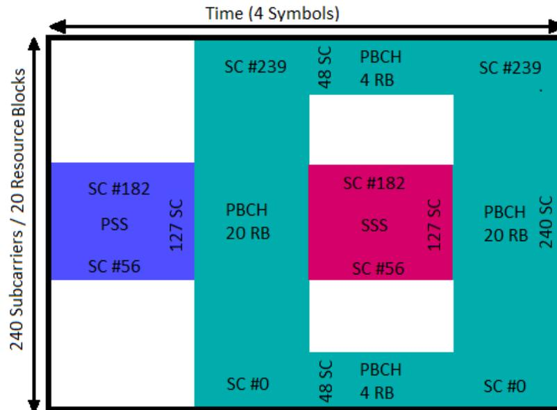
Figure 2. Structure of SSB [8].
