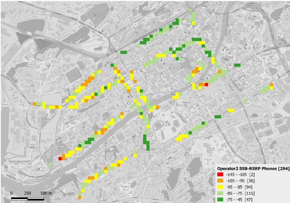
Figure 32. Operator2 SSB-RSRP of phones in September 2020.
