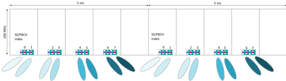
Figure 3. SSB transmitted on different spatial beams [8].
