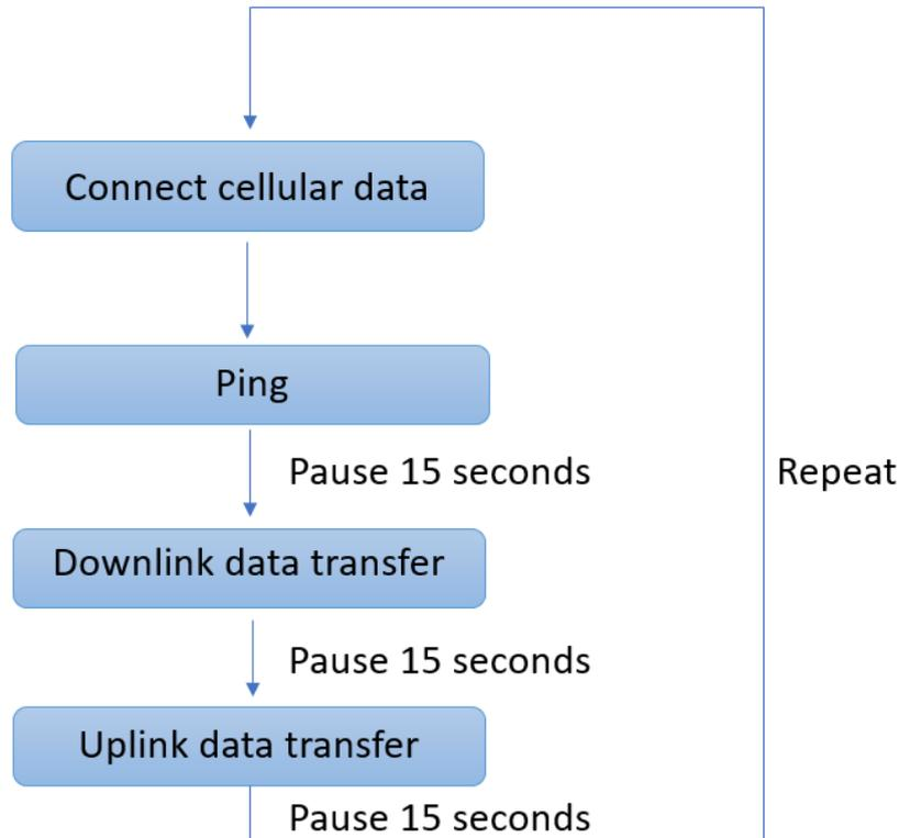
Figure 9. Block diagram of the measurement script.
