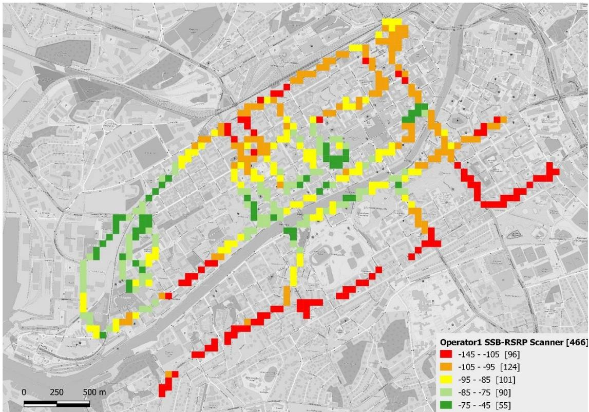
Figure 18. Operator1 SSB-RSRP of scanner in May 2020.
