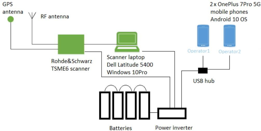
Figure 7. Measurement equipment setup.
