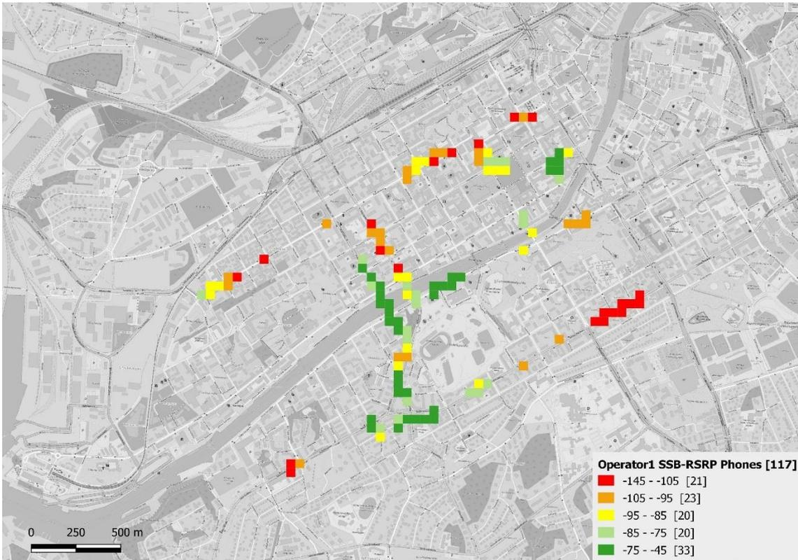
Figure 30. Operator1 SSB-RSRP of phones in September 2020.
