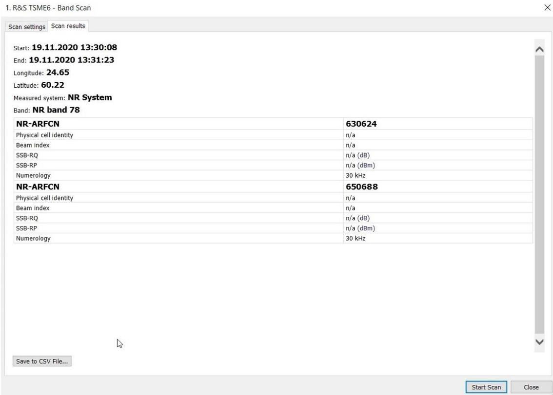
Figure 8. Example of band scan results with TSME6 scanner.
