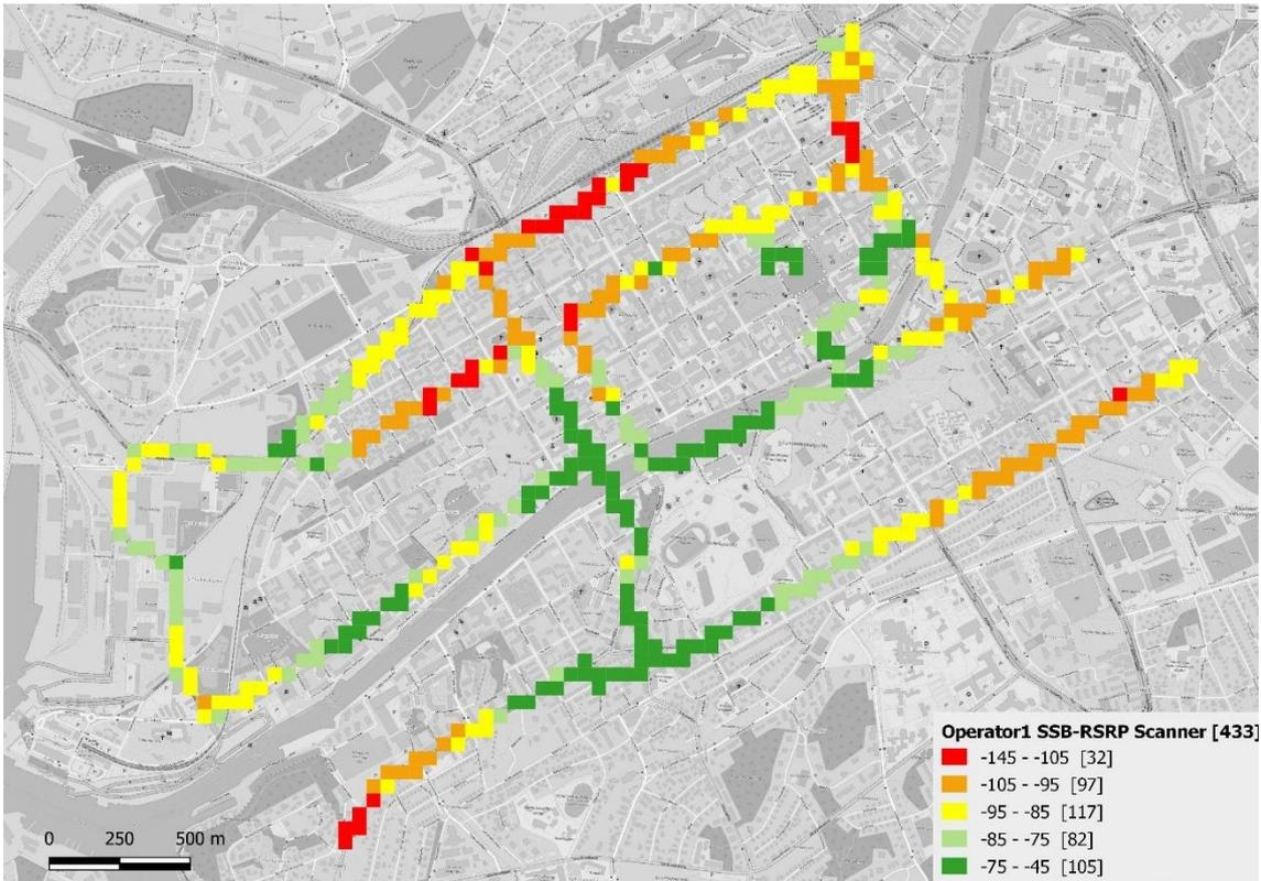
Figure 19. Operator1 SSB-RSRP of scanner in September 2020.
