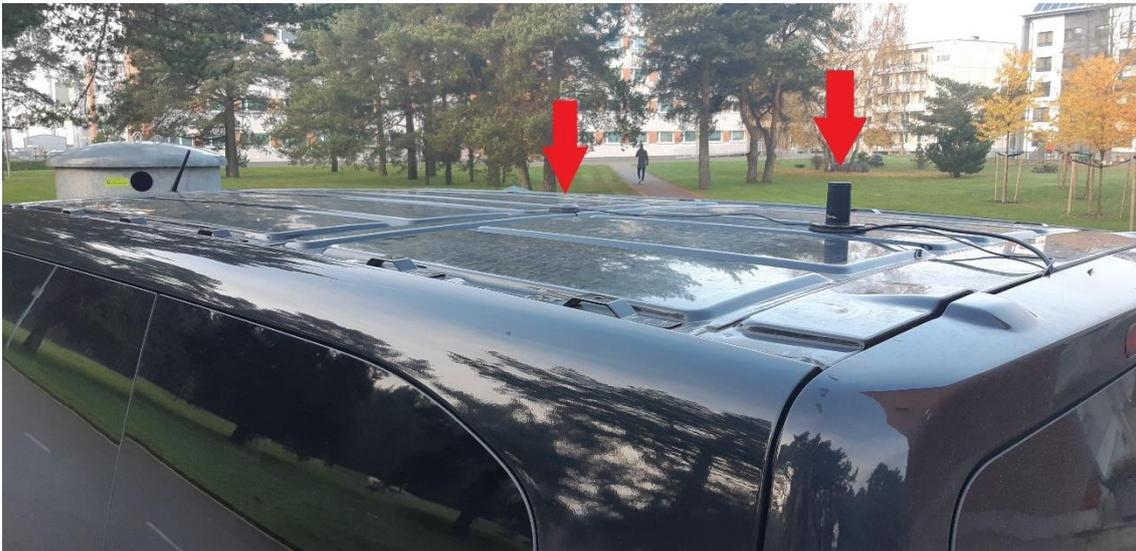
Figure 5. GPS (left) and RF (right) antenna of the scanner on the roof of measurement bus.
