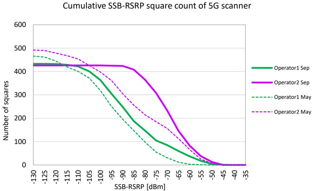
Figure 15. Cumulative square count of scanner in May (solid line) and in September (dashed line).
